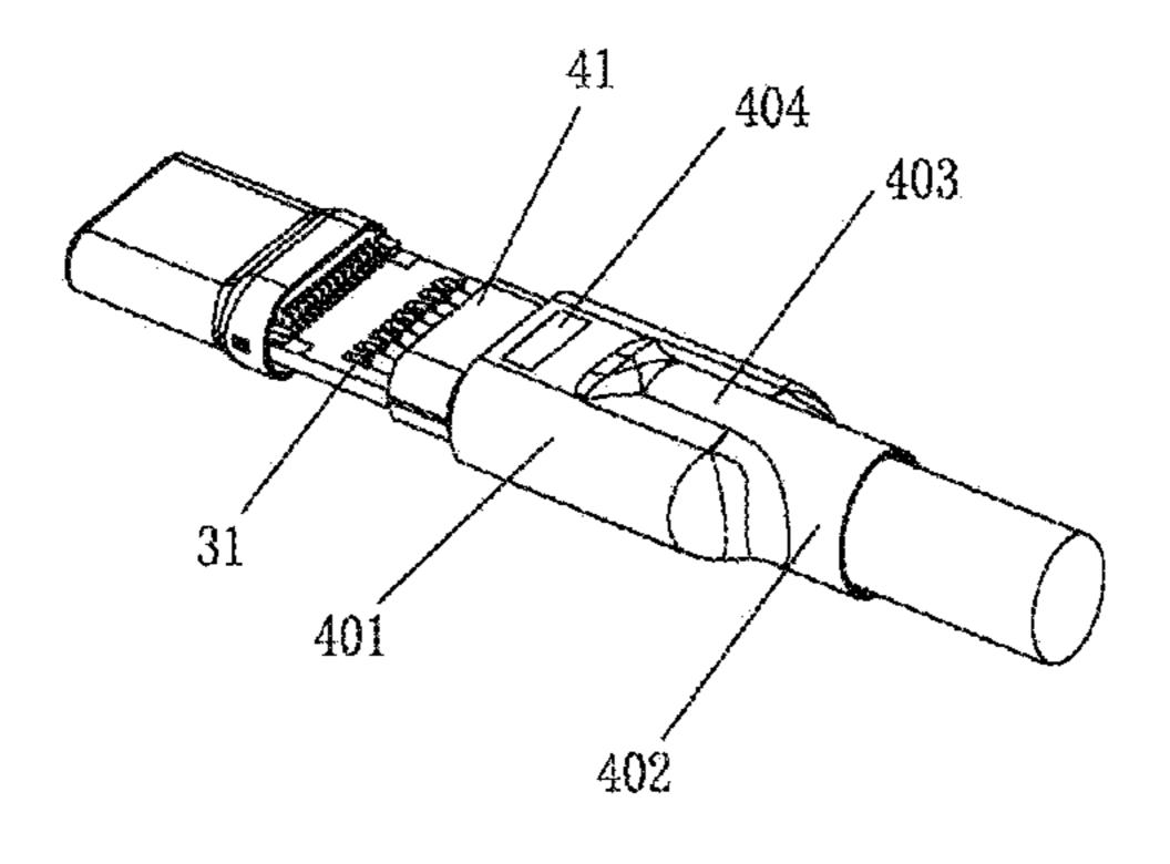
disposed between the first surface and the second surface, and the shielding plate includes a protrusion which is extended out of a side of the base and abuts against the second metal shell. As a result, a new grounding path is formed, which can reduce the electromagnetic interference and strengthen the insulating effect.
