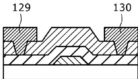
FORMATION OF SOURCE ELECTRODE AND DRAIN ELECTRODE (SECOND WIRING)
