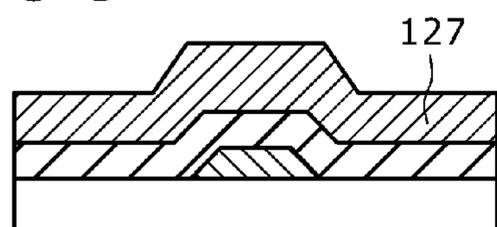
DEPOSITION OF INSULATING FILM ( $\text{SiO}_2$ )
