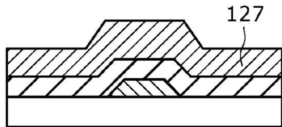
DEPOSITION OF INSULATING FILM ( $\text{SiO}_2$ )
