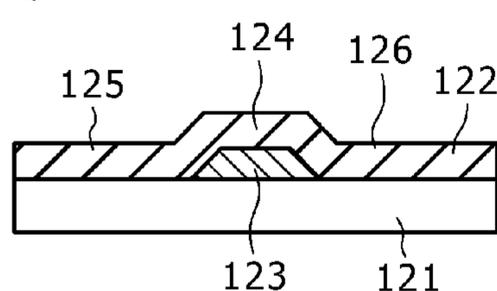
FORMATION OF GATE INSULATING FILM ( $\text{SiO}_2$ ) DEPOSITION AND POLYCRYSTALLIZATION OF AMORPHOUS Si FORMATION OF SOURCE AND DRAIN
