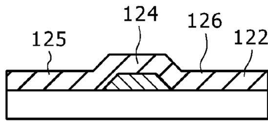
FORMATION OF GATE INSULATING FILM ( $\text{SiO}_2$ ) DEPOSITION AND POLYCRYSTALLIZATION OF AMORPHOUS Si FORMATION OF SOURCE AND DRAIN
