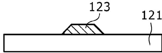
FORMATION OF GATE ELECTRODE (FIRST WIRING)
