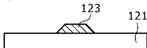
FORMATION OF GATE ELECTRODE (FIRST WIRING)
