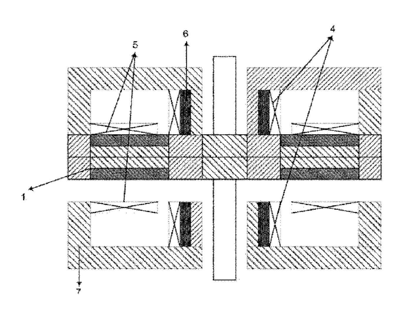
a permanent magnetic holding component to hold the movable unit in the first position or the second position. The magnetic actuator can simplify the actuator, reduce the number of components and the size thereof, as well as reducing the energy consumption and improving the stability thereof.
