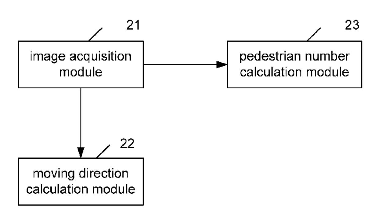
edge points of pedestrian images are extracted from a foreground image of the current frame image, and performing joint weighted counting on the edge points of the pedestrian images and the moving feature points of the current frame image according to correction coefficients of locations of the respective points, to obtain the number of the pedestrians. A device for calculating the number and moving direction of pedestrians is also provided.
