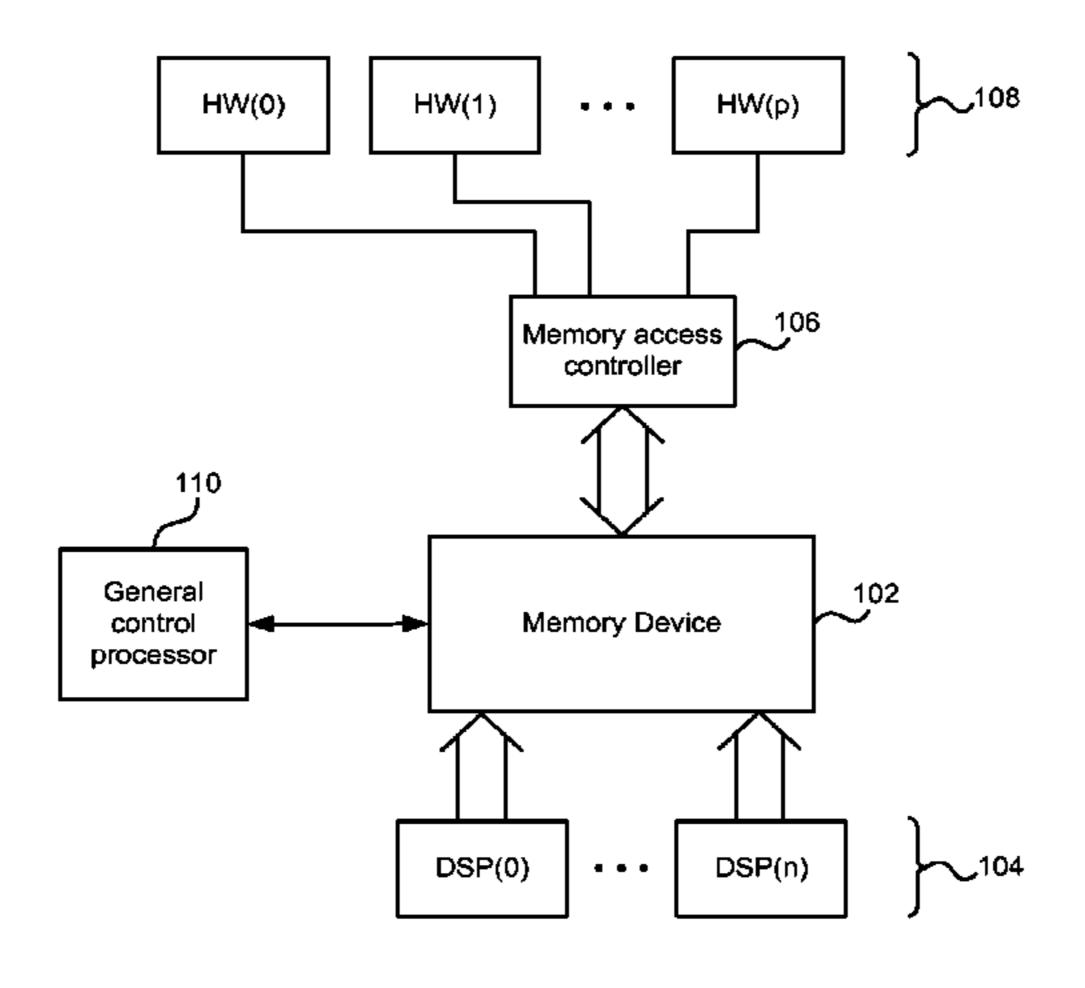
allocated to a memory access channel, and the threads are configured to detect an occurrence of an event and, responsive to this, control the memory access controller to enable a selected fixed function accelerator to read data from or write data to the memory device via its memory access channel.
