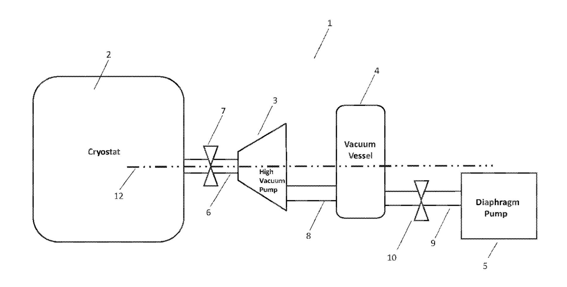
suitable pressure range. This removes the need for the output of the high-vacuum pump to be connected to a continuously operating, second-stage vacuum pump. Furthermore, the second vacuum pump is only required to be operated periodically in order to maintain the pressure in the vacuum vessel below the threshold pressure.
