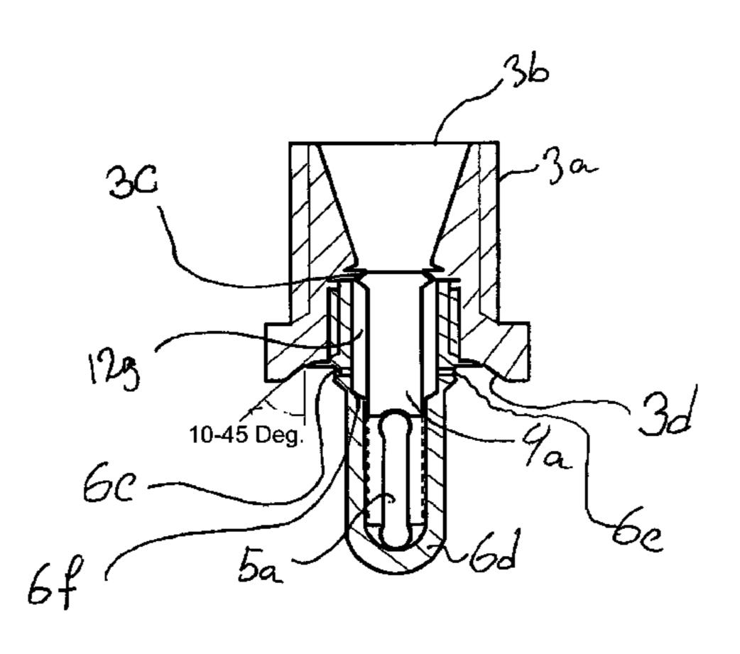
and deflecting surface (3d, 12d) have a mutual positioning so that straight liquid jets flowing through the bores (6c, 9c) will hit the deflecting surface (3d, 12d) with at least a bevel angle  $\alpha$ .
