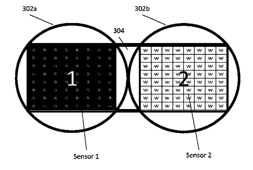
scaling difference and a sharpness difference between the color and luminance images, the scaling and sharpness differences being due to the AF mechanism, and to process the color and luminance images into a fused color image using the calculated differences.
