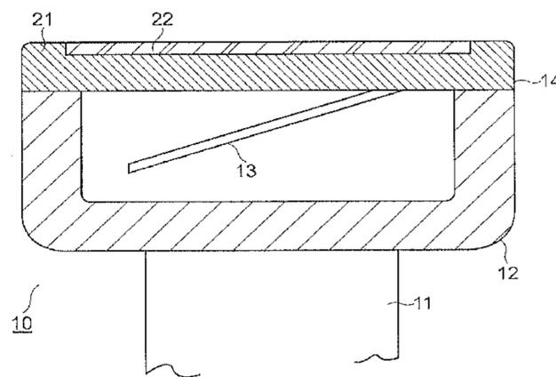
member being formed of a material, which is highly compatible with the central member, shows excellent interruption performance and had high withstand voltage, and being provided outside the central member and fixed thereto.
