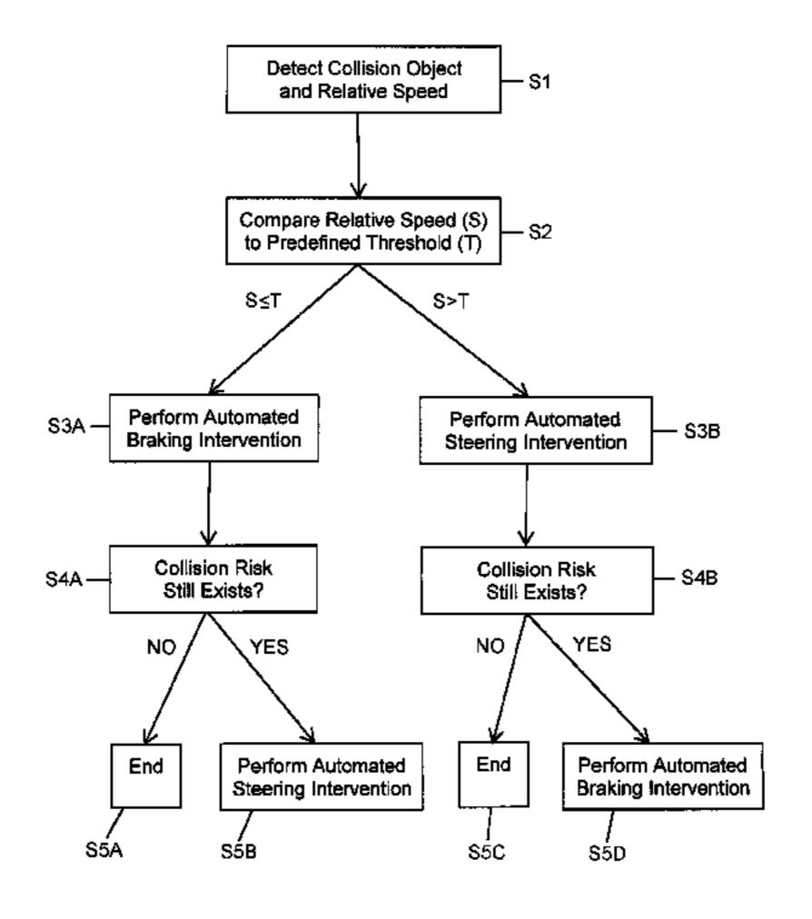
vehicle's surroundings, and a relative speed of the vehicle relative to the potential collision object. The activation and/or the sequence of an automated steering intervention and/or an automated braking intervention is determined based on the relative speed. The braking intervention is activated at first when the relative speed is below or equal to a predefined threshold, and the steering intervention is activated at first when the relative speed is above the predefined threshold.
