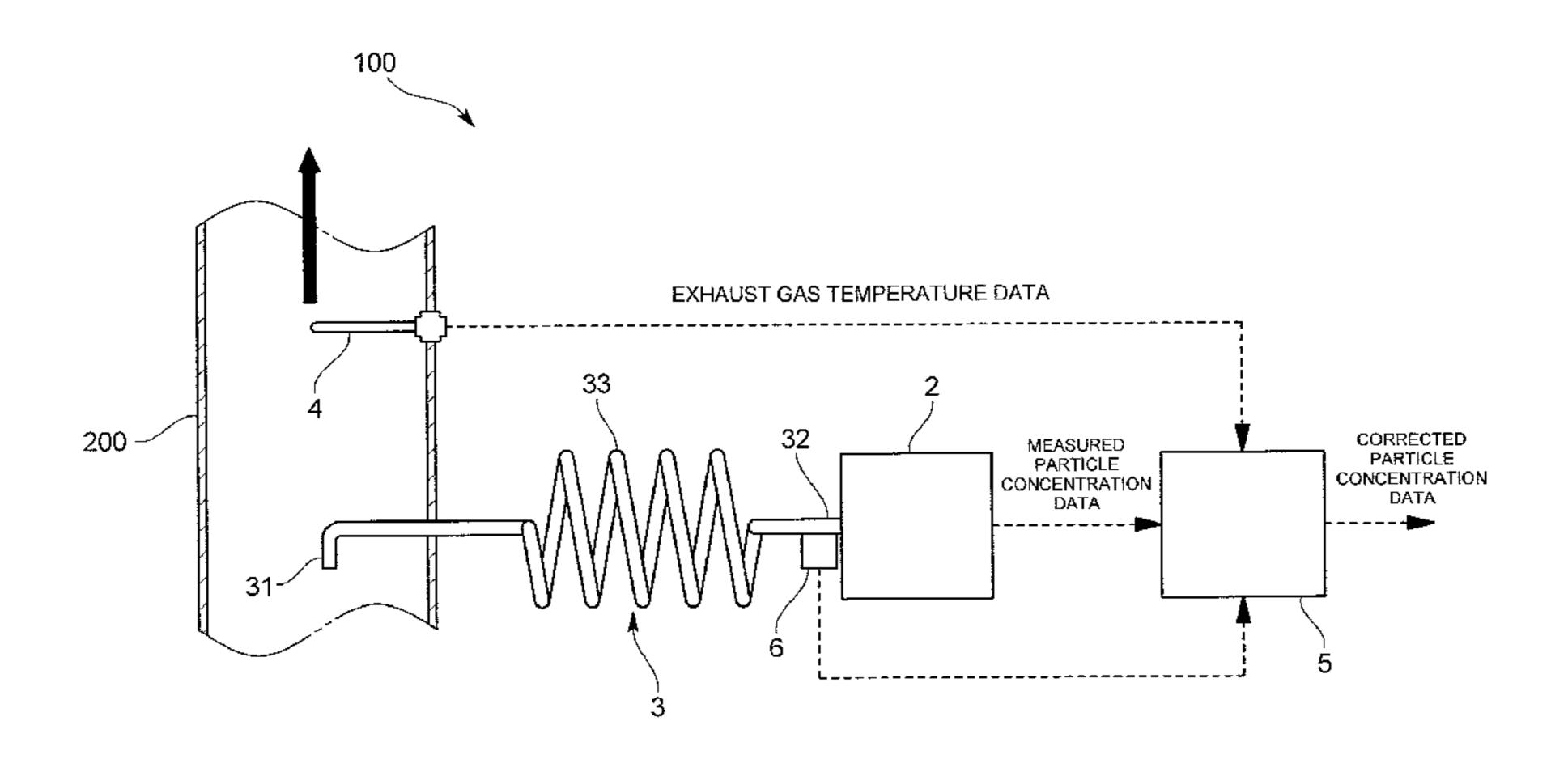
ment device in real time to calculate the particle concentration of the exhaust gas flowing through the exhaust gas transfer pipe.
