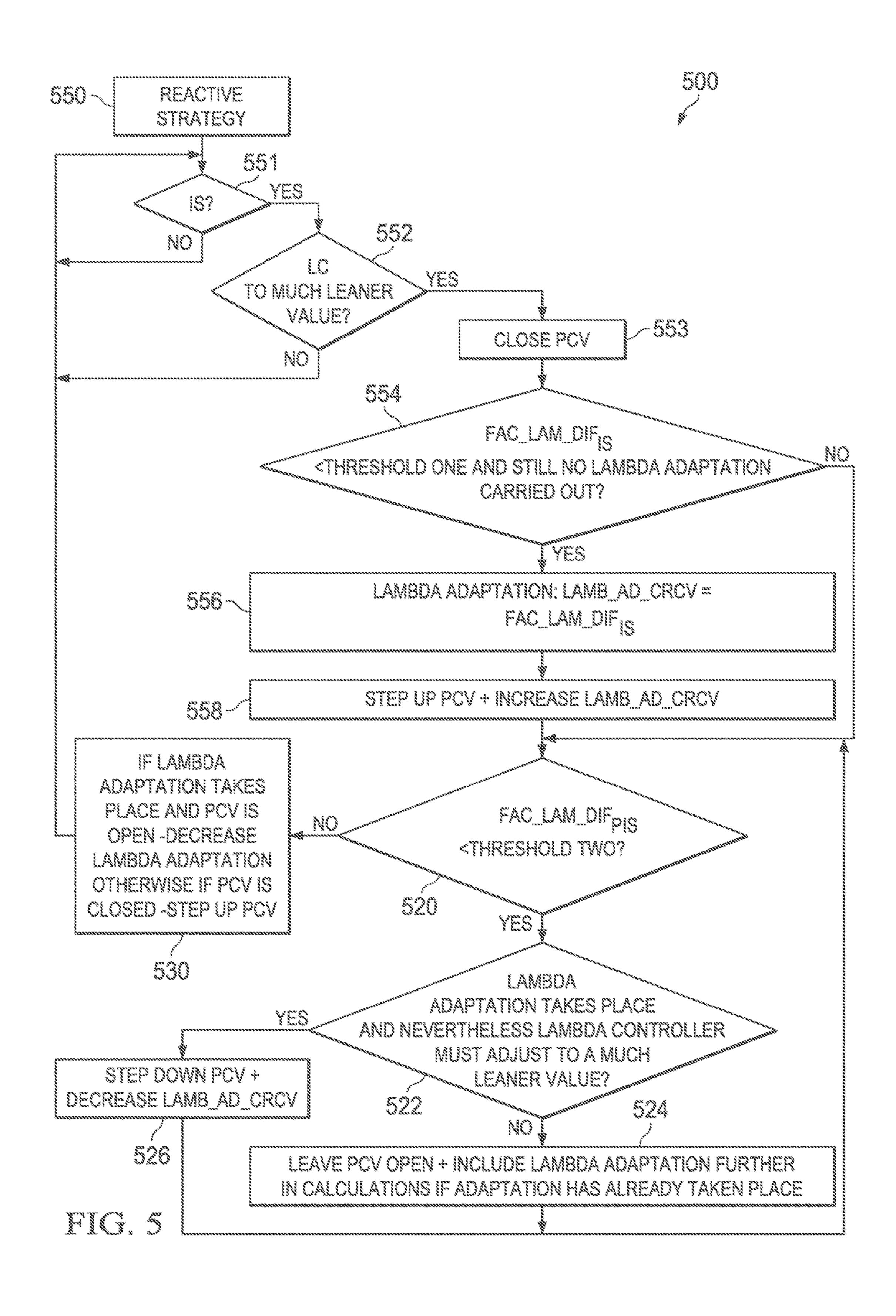
DETERMINING OUTGASSING OF A FUEL FROM A LUBRICANT WITHIN AN INTERNAL COMBUSTION ENGINE AND LAMBDA VALUE ADAPTATION BASED ON THE DETERMINED OUTGASSING OF FUEL
