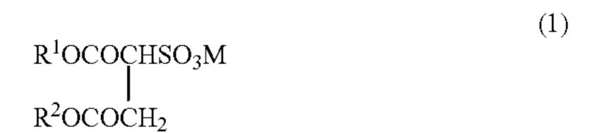
wherein R<sup>1</sup> and R<sup>2</sup> are the same as or different from each other, and each represent a  $C_4$  to  $C_{12}$  non-fluorinated saturated hydrocarbon group; and M is an alkali metal, an ammonium salt, or an amine salt,
