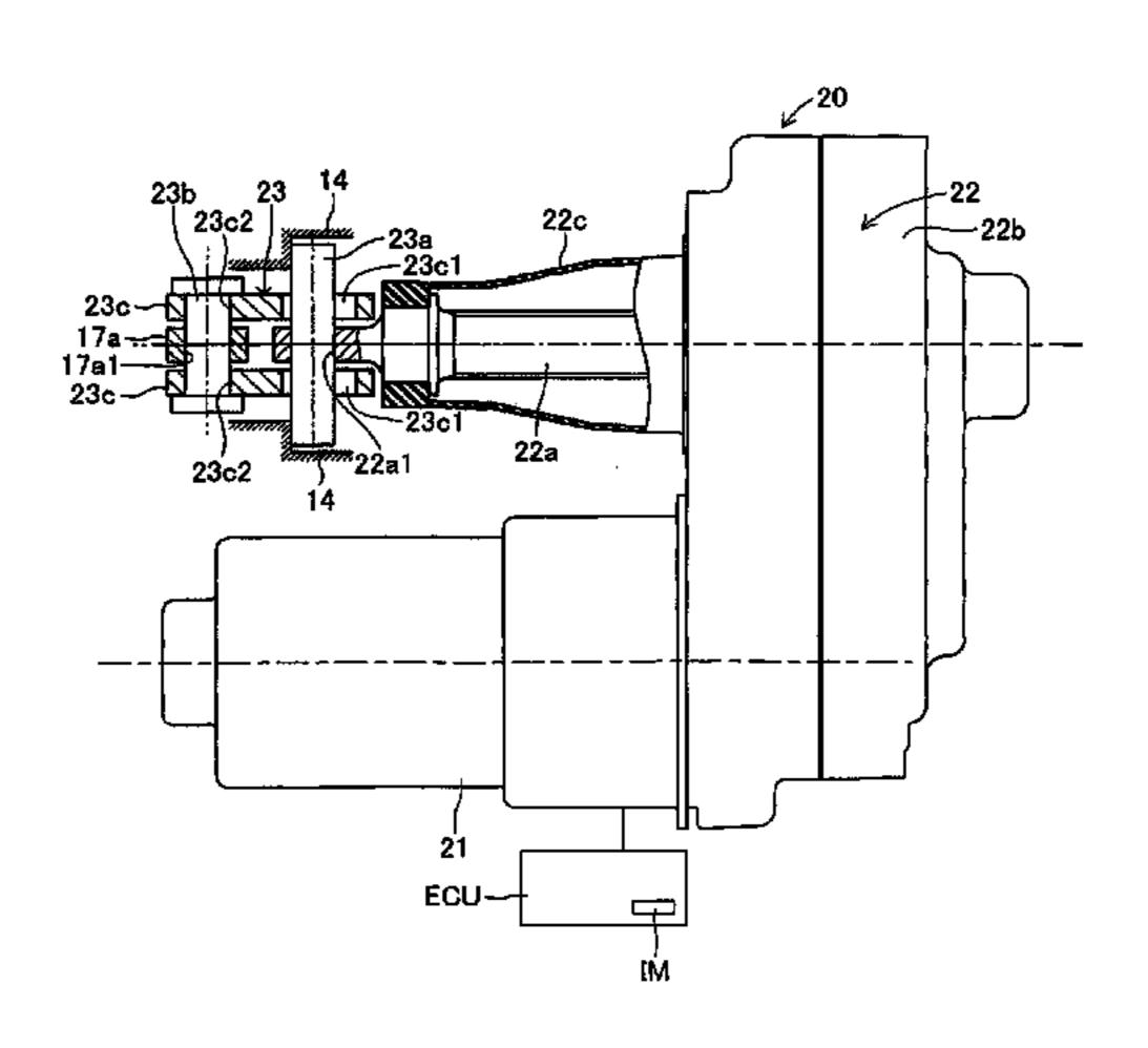
connection pin. A connection member is rotatable with respect to the end of the shaft member in the circumferential direction of the first connection pin at a first hole where the connection member is fitted on the first connection pin, is rotatable with respect to the parking lever in the circumferential direction of the second connection pin at a second hole where the connection member is fitted on the second connection pin, and connects the two pins.
