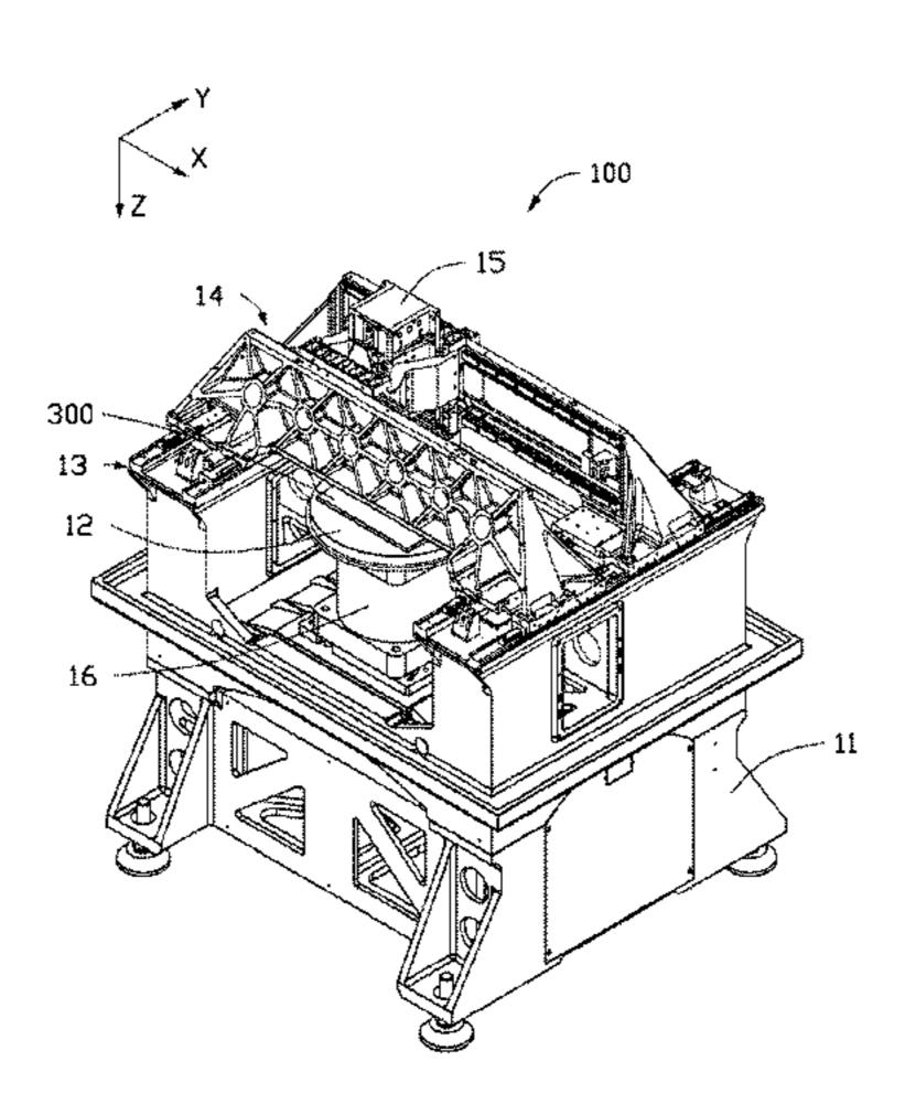
module drives the feeding module to move along a second direction perpendicular to the first direction. The cutter is positioned on the feeding module. The feeding module is capable of driving the cutter to move back and forth along a third direction under the control of the control module. The third direction is perpendicular to first and second direction.
