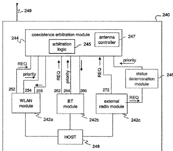
coexistence arbitration module may be a separate module or may be integrated into another module or distributed among the modules. The device may include a host processor for altering transmission characteristics of a module to increase the likelihood that another module can receive data within a reasonable time period.
