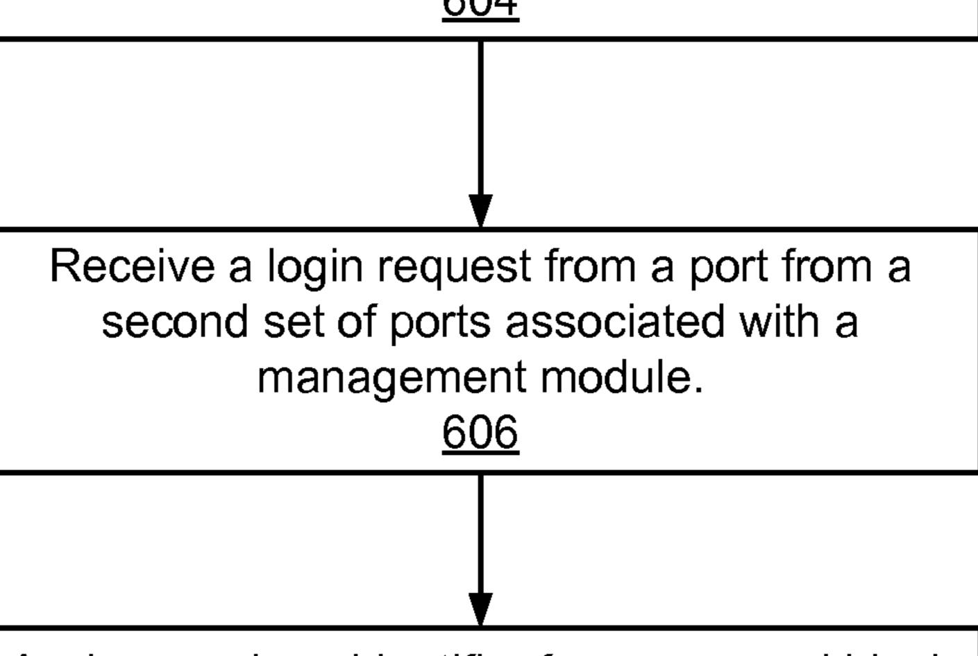
Assign a unique identifier from a second block of identifiers to the port from the second set of ports in response to the login request received from that port from the second set of ports.
