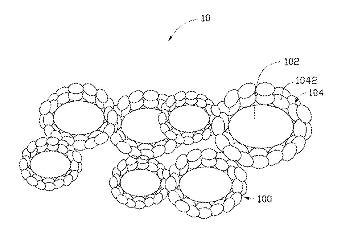
particles are mixed to form a lithium iron phosphate precursor slurry. Outer surfaces of the lithium vanadium phosphate particles are coated with the lithium iron phosphate precursor.
