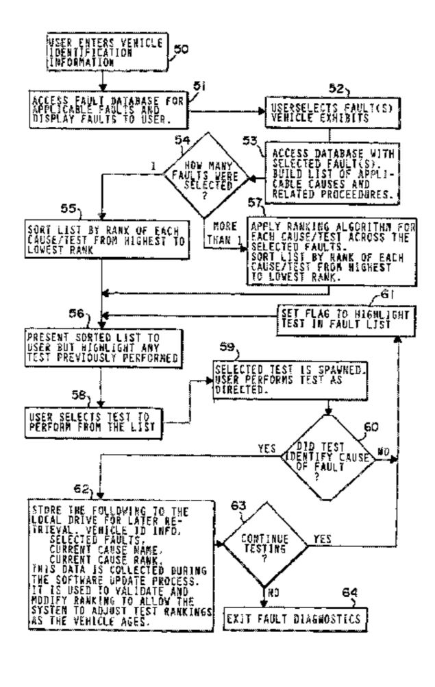
procedures may include links to the engine analyzer or scanner hardware or other appropriate test modules.
