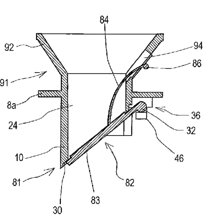
fitted to the carrier member, the biasing portion is elastically deformed and biases the cover portion to thereby bring the cover portion into contact with a seat portion provided at an end of the through hole of the carrier member.
