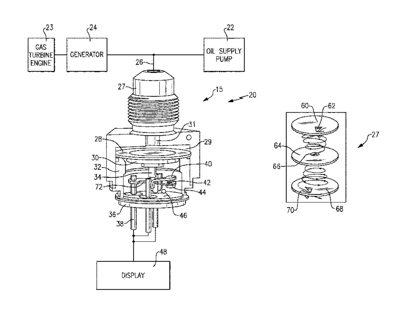
pressure in the pressure chamber to cause contact between a moveable contact and a fixed contact. An orifice communicates a fluid pressure into the pressure chamber. The orifice provides a tortuous path for a fluid flow to reach the pressure chamber. An oil supply system and a generator are also disclosed.
