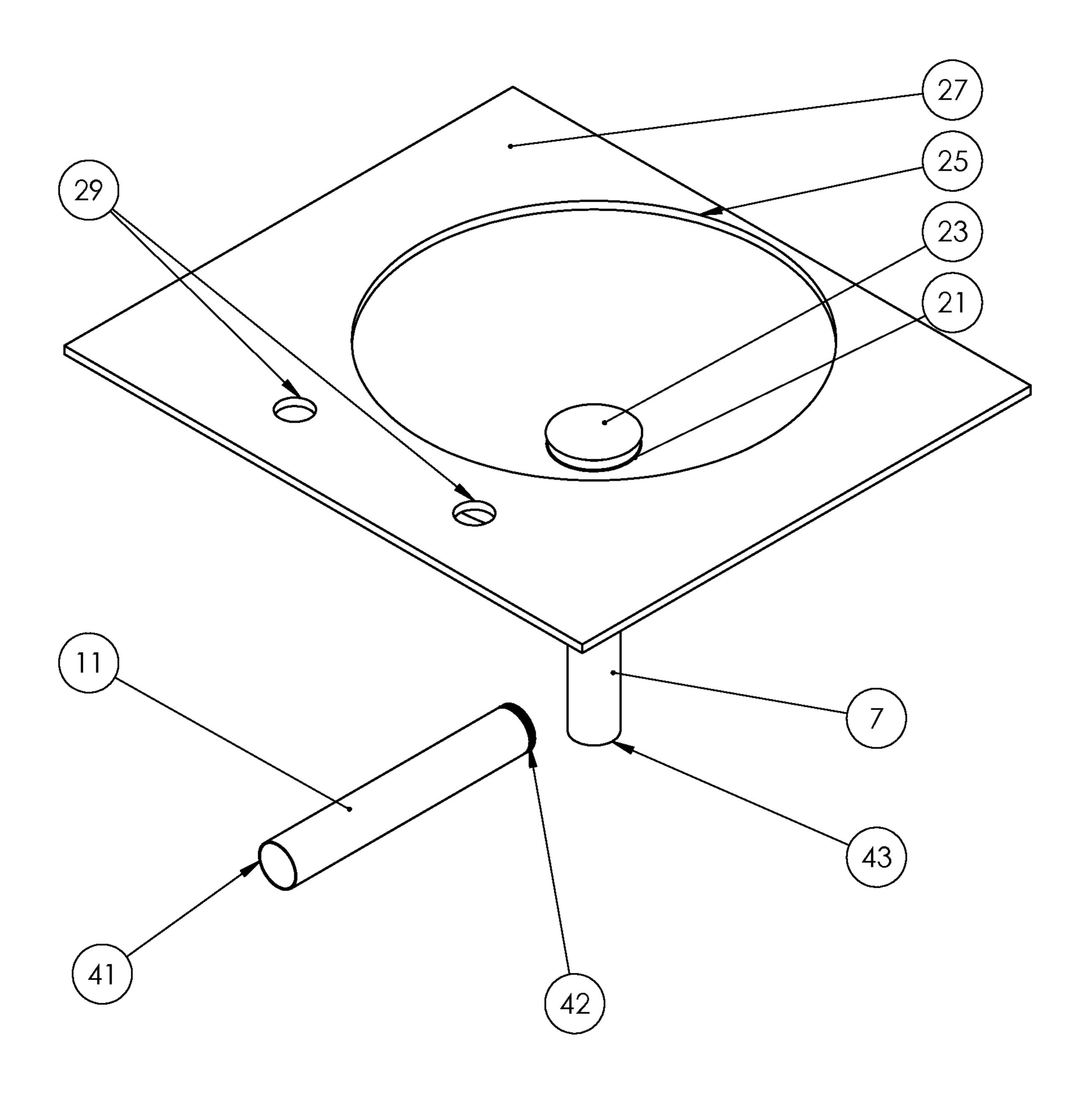
Fig. 4. Isometric view of a lavatory sink showing vertical tailpiece and disconnected horizontal waste arm.
