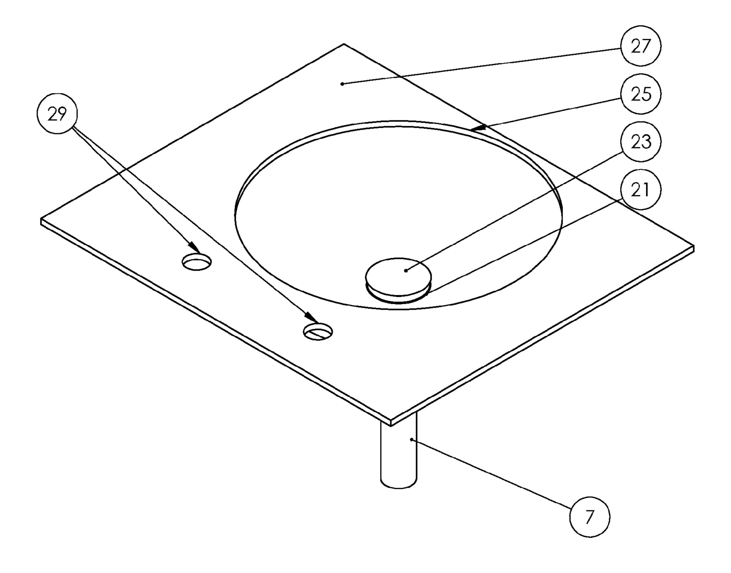
Fig. 3. Isometric view of a lavatory sink equipped with a lavatory drain fitting ending in a vertical tubular tailpiece.
