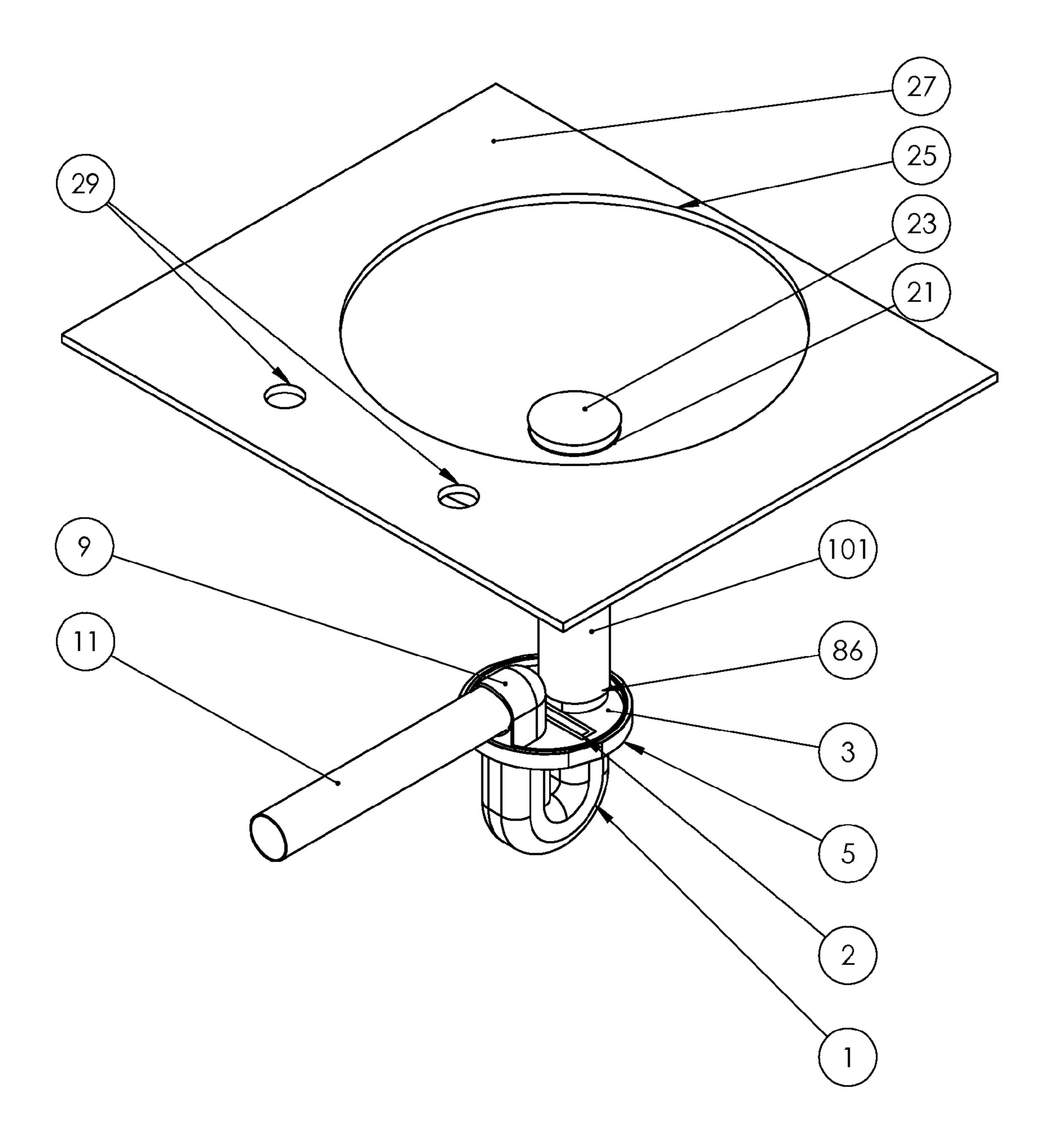
Fig. 10. Isometric view of removable trap system showing securing nuts.
