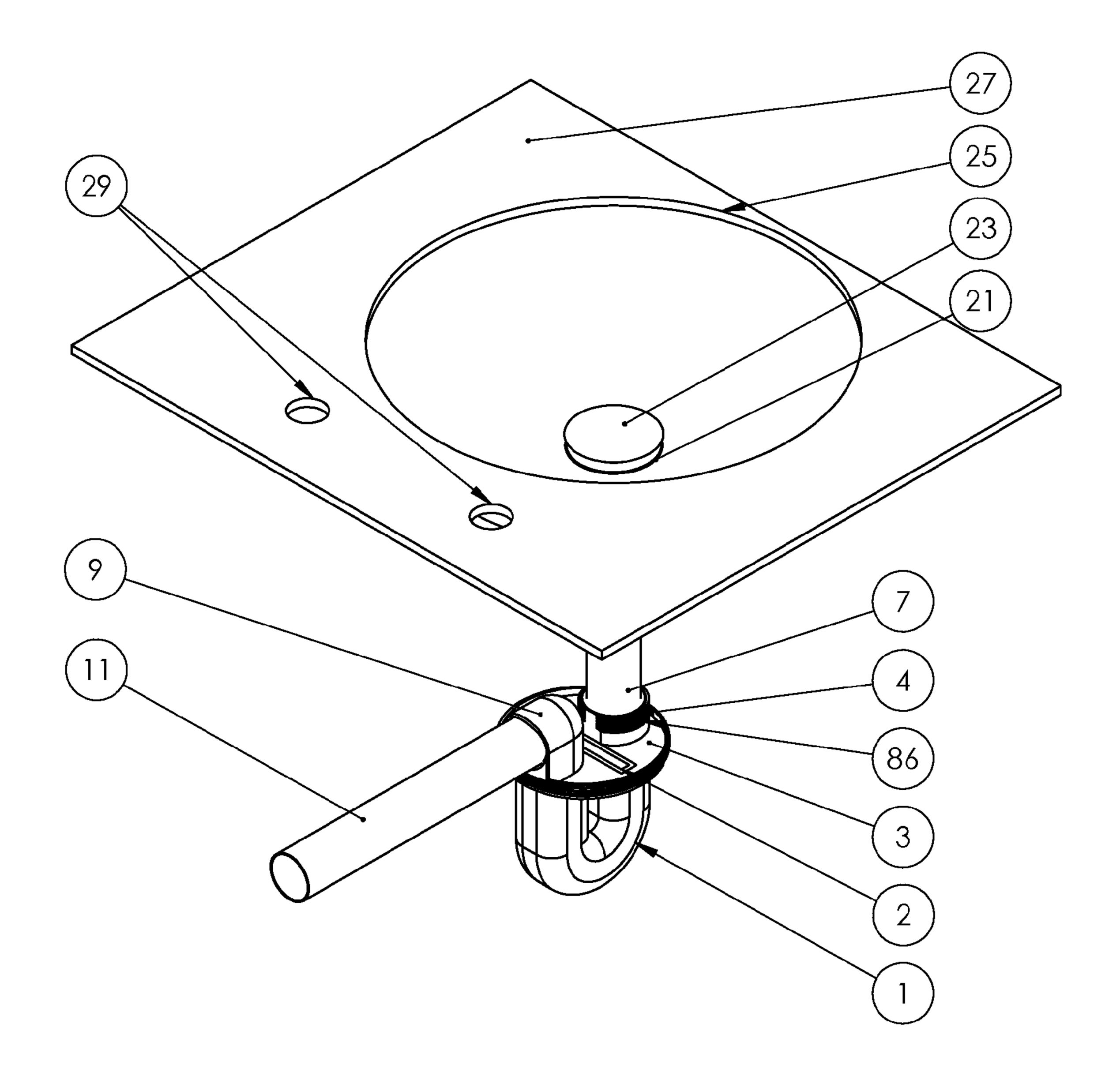
Fig. 8. Isometric view of removable trap system showing drain, tailpiece, waste arm, trap, seals, and connecting top.
