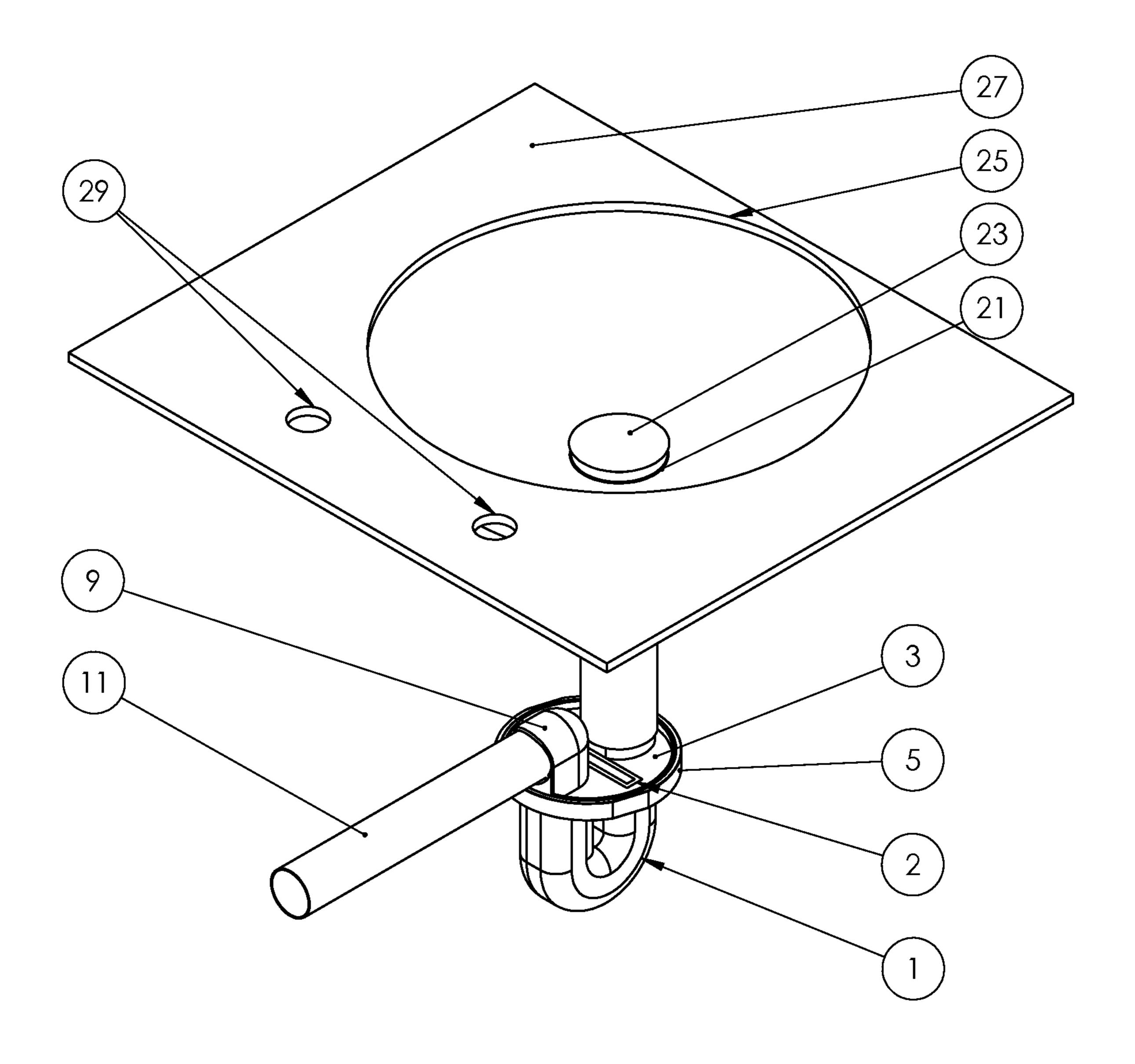
Fig. 1. Isometric view of removable trap system attached to the underside of a lavatory sink fitting.
