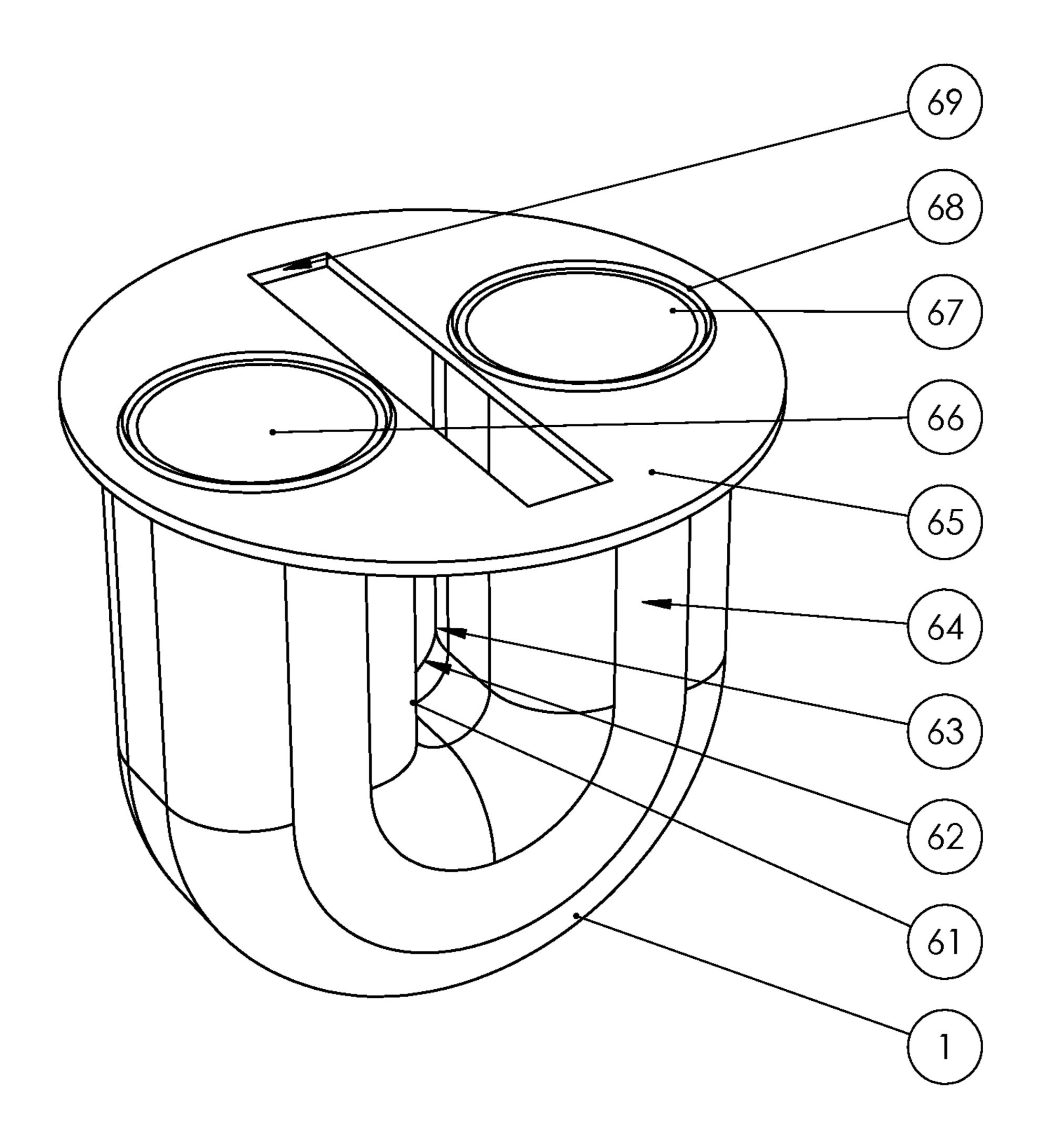
Fig. 6. Isometric view of the removable U-bend trap cartridge.
