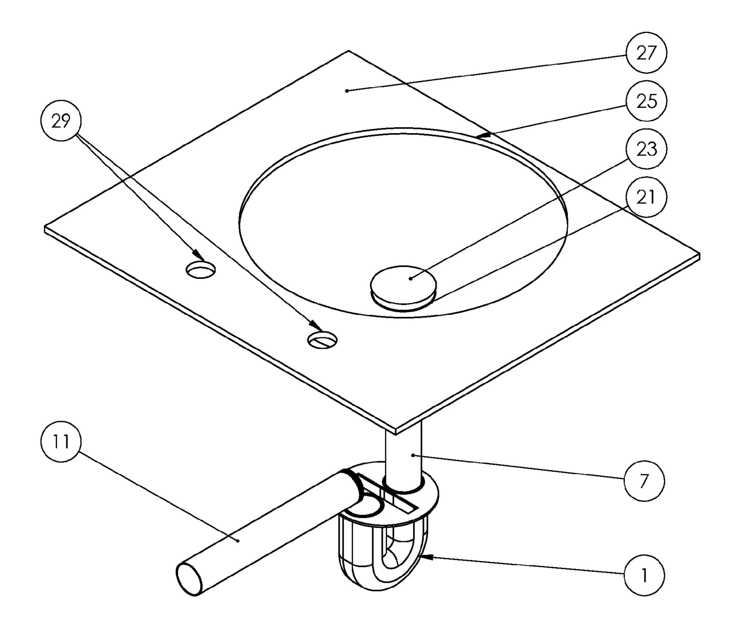
Fig. 5. Isometric view of removable trap system showing drain, tailpiece, waste arm, and tubular trap portion.
