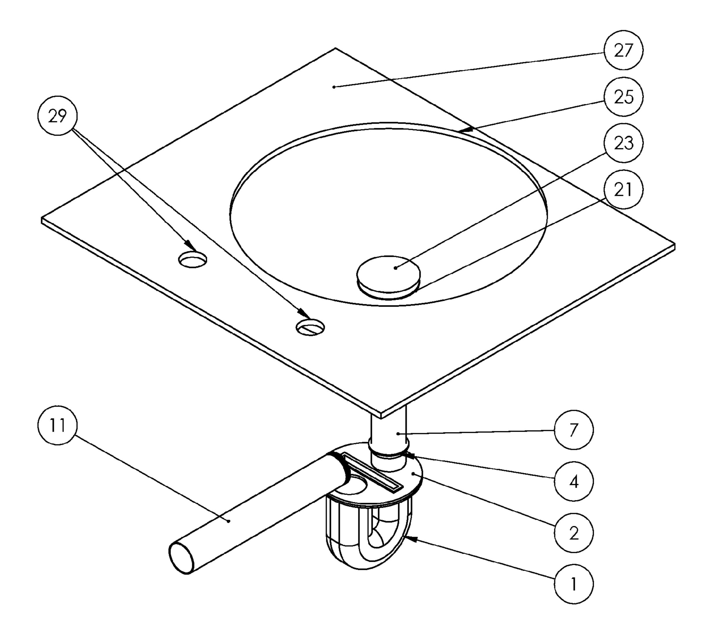
Fig. 7. Isometric view of removable trap system showing drain, tailpiece, waste arm, tubular trap, and seals.
