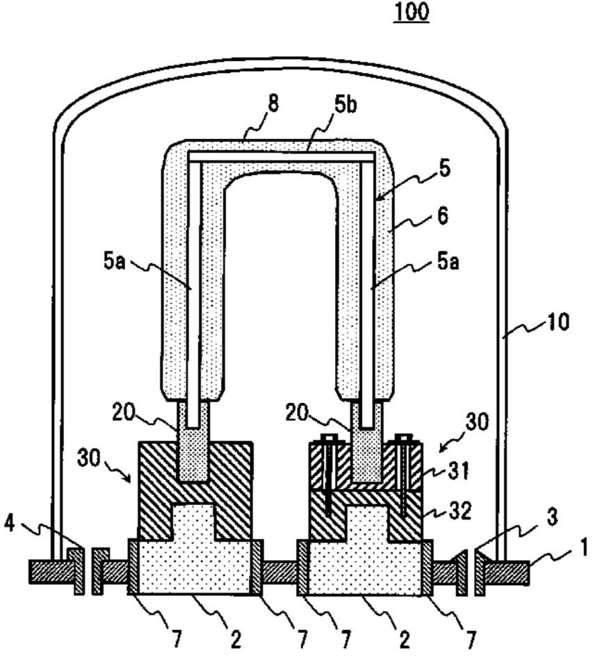
lower electrode 32 in contact with the lower surface 34 of the upper electrode 31 in FIG. 2) that is a contact surface with an upper surface of the lower electrode 32, thereby providing an effect of preventing occurrence of a crack or a break in a U rod that can be expanded and contracted in all directions during a vapor phase growth process.
