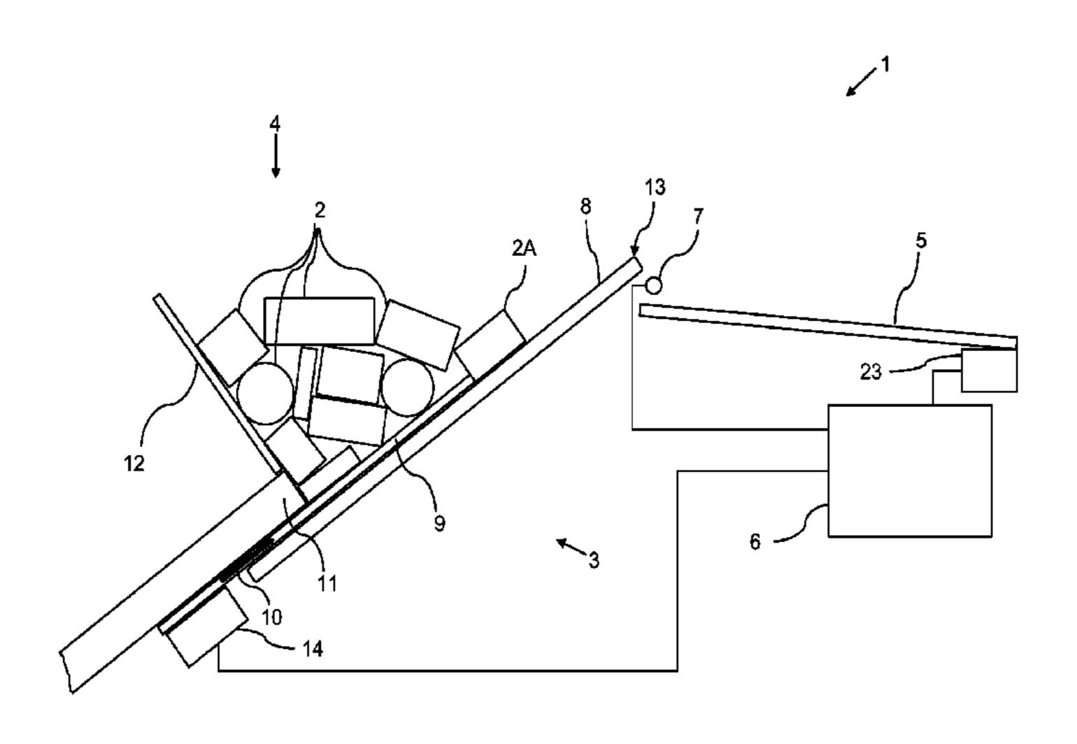
stepped conveyor, which control device is coupled to a sensor which detects whether a piece goods item has been conveyed beyond the upper edge.
