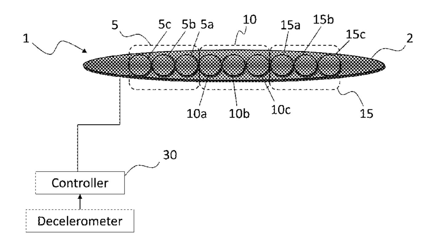
(c) an illumination state in which increasing numbers of the plurality of lights of each of the at least two outer sections are progressively illuminated in response to corresponding and progressively increasing amounts of vehicle deceleration above a predetermined threshold.
