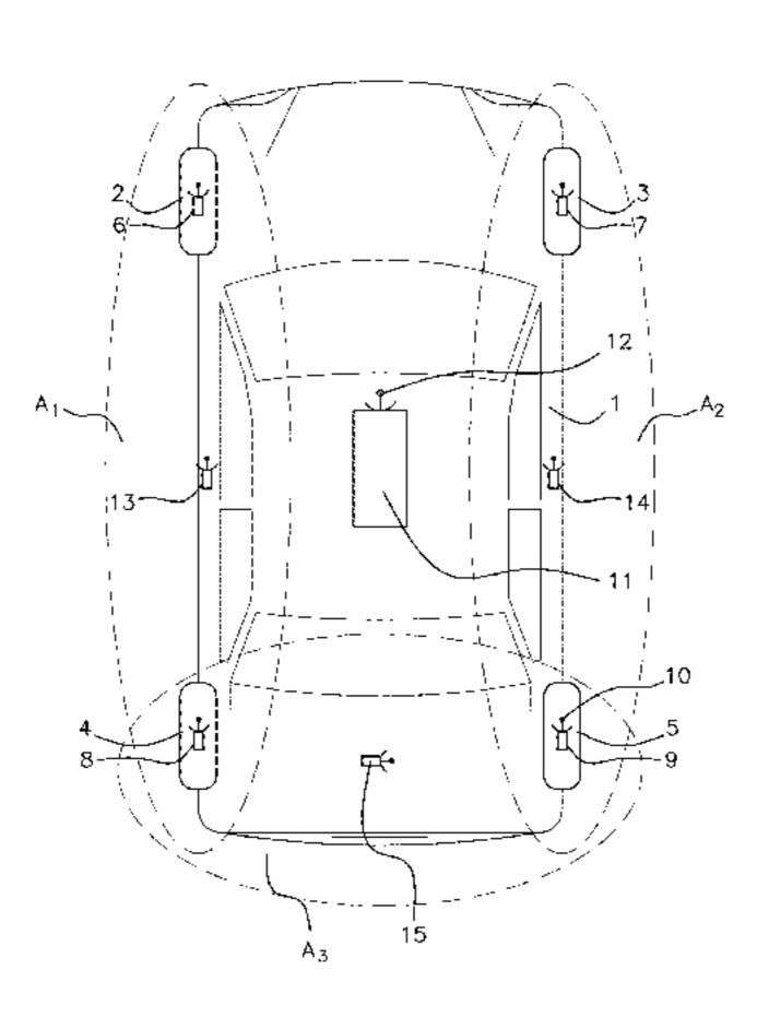
fitted to the vehicle, using as the criterion for determining this "actual position"  $\overrightarrow{WU}_i$  the rate of reception, by the electronic module, of the signals transmitted by each transmitting antenna.
