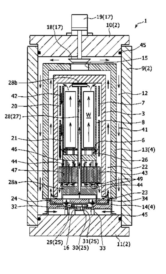
circulation flow (41). In the cooling promotion flow path (44), the pressure medium gas that is in the second circulation flow (42) and that has performed heat exchange with the object-of-processing (W) is guided to the heat accumulator (43) and cooled by the heat accumulator (43) before the pressure medium gas merges with the first circulation flow (41).
