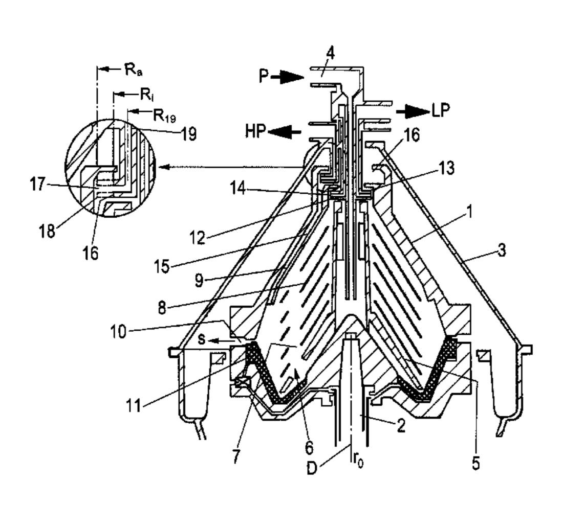
to discharge a solids phase from the drum. A separation zone is formed between the lighter phase and the heavier phase in the separator.
