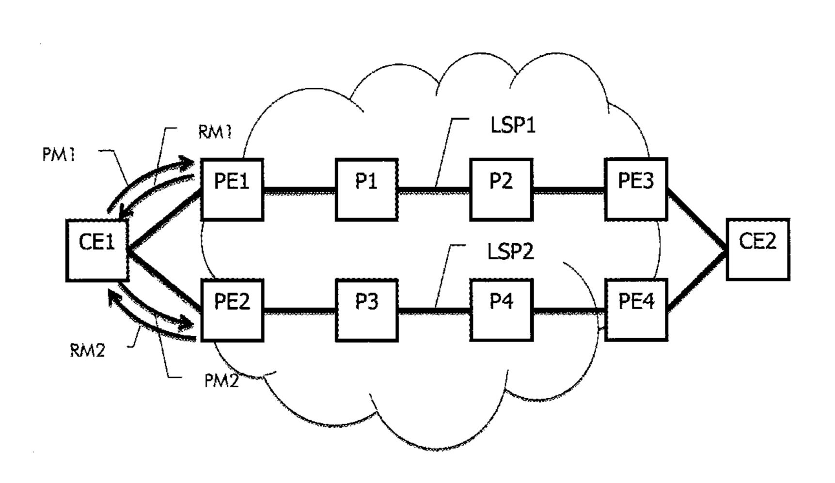
through the provider network to be established from a second provider edge node and to be disjoint from said first traffic path, the customer edge device forwards the data element to the second provider edge node to enable path calculation of the second traffic path using the shared constraint information as exclusion list.
