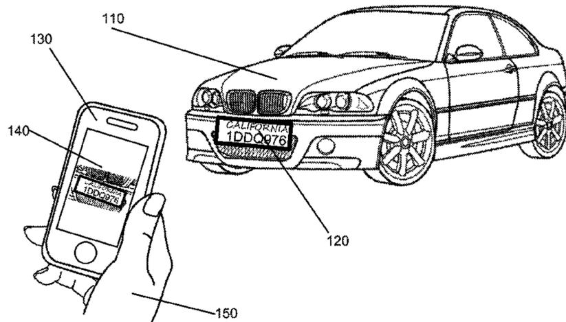
includes a license plate detector configured to process the electrical signal to recover information from the vehicle license plate image. The mobile apparatus includes an interface configured to transmit the vehicle license plate information to a remote apparatus and receive a location of a vehicle service center corresponding to the vehicle license plate image in response to the transmission.
