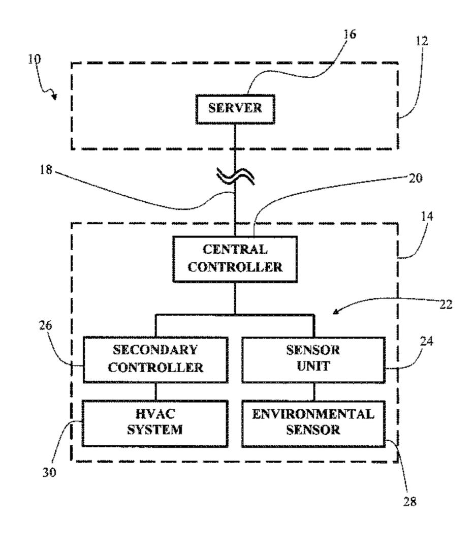
to operate the HVAC systems. The invention includes the method of providing tailored HVAC related controls, reports, notices and diagnostic services to a client under various subscription plans.
