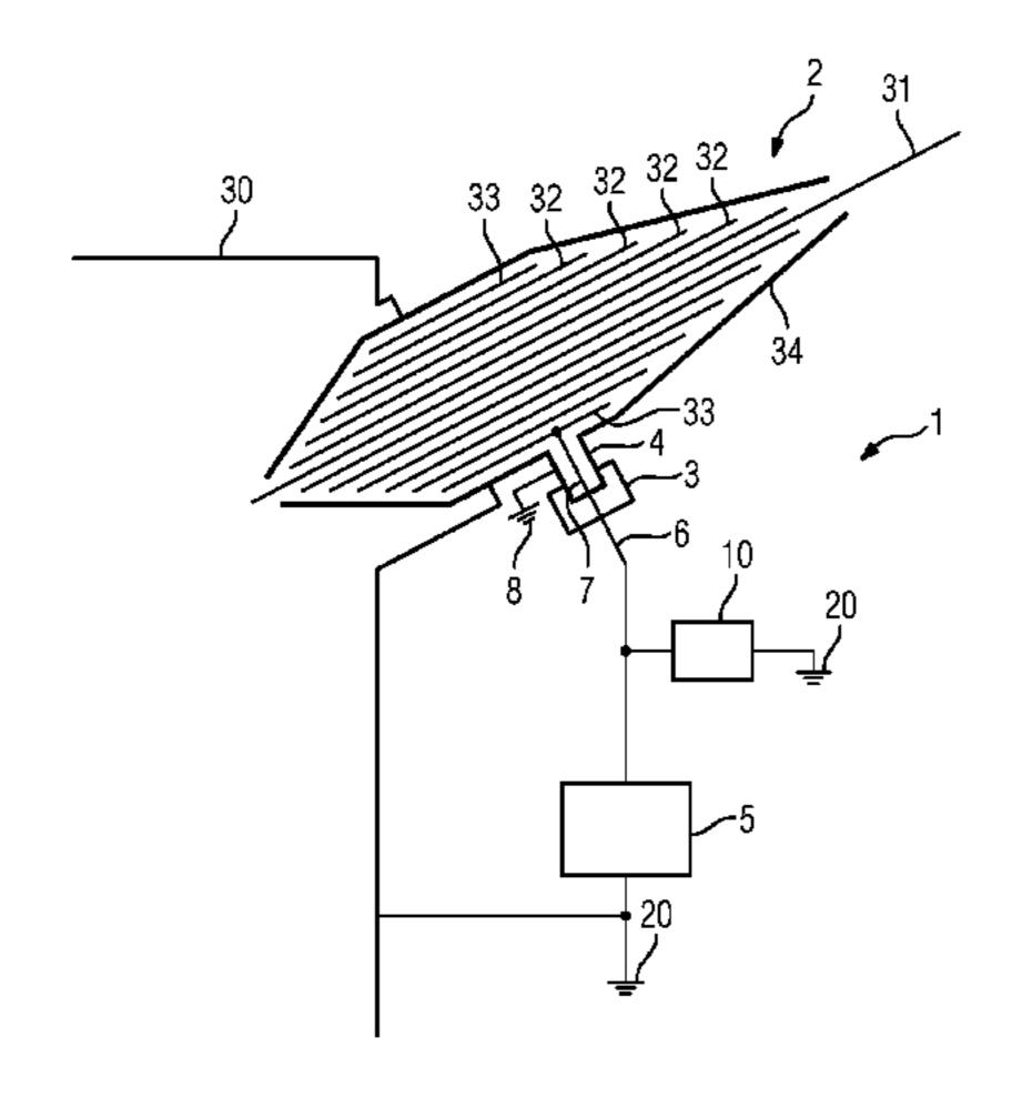
stage responds to overvoltages at operating frequency, the second stage responds to high-frequency overvoltages. A third protective stage is connected between the measurement connection and the first protective stage in parallel with the measurement connection and includes a mechanical switch for short-circuiting when a third response voltage is present.
