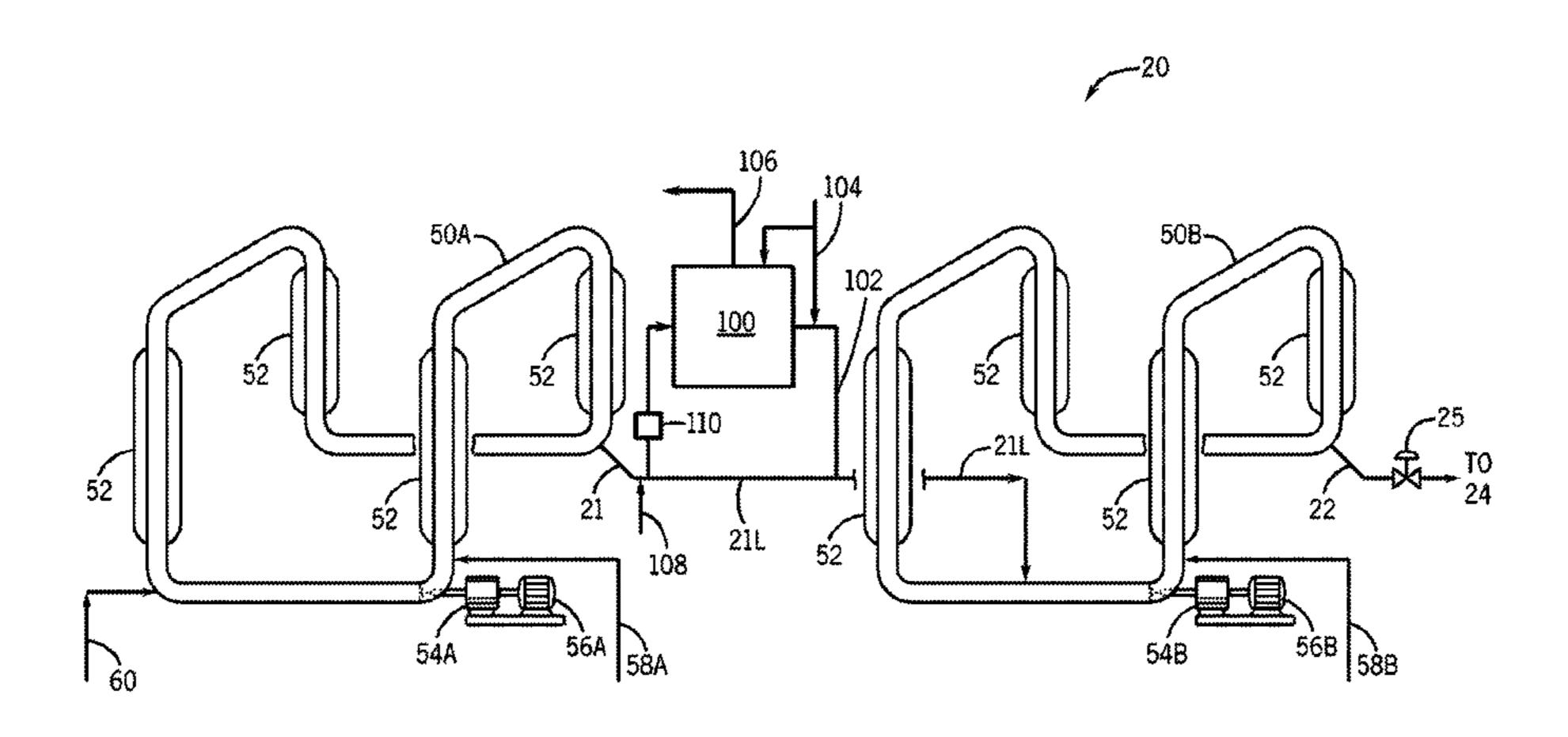
olefin in the second reactor to form a second polyolefin, and discharging from the second reactor a slurry having the second polyolefin.
