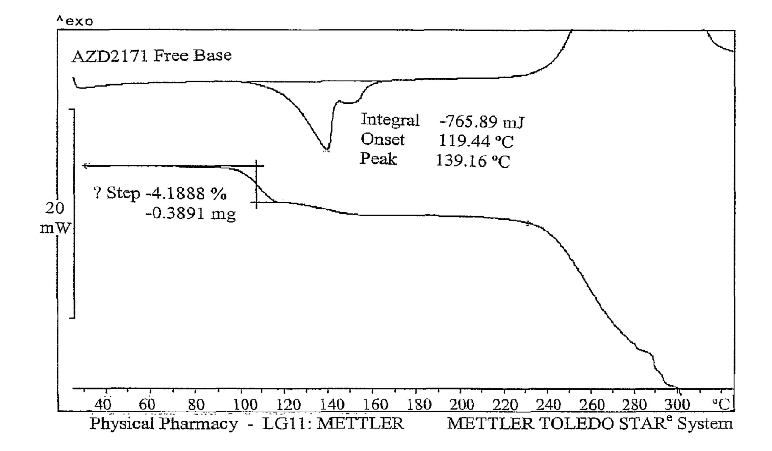
Figure 1: DSC and TGA Thermograms AZD2171 Free base Monohydrate
