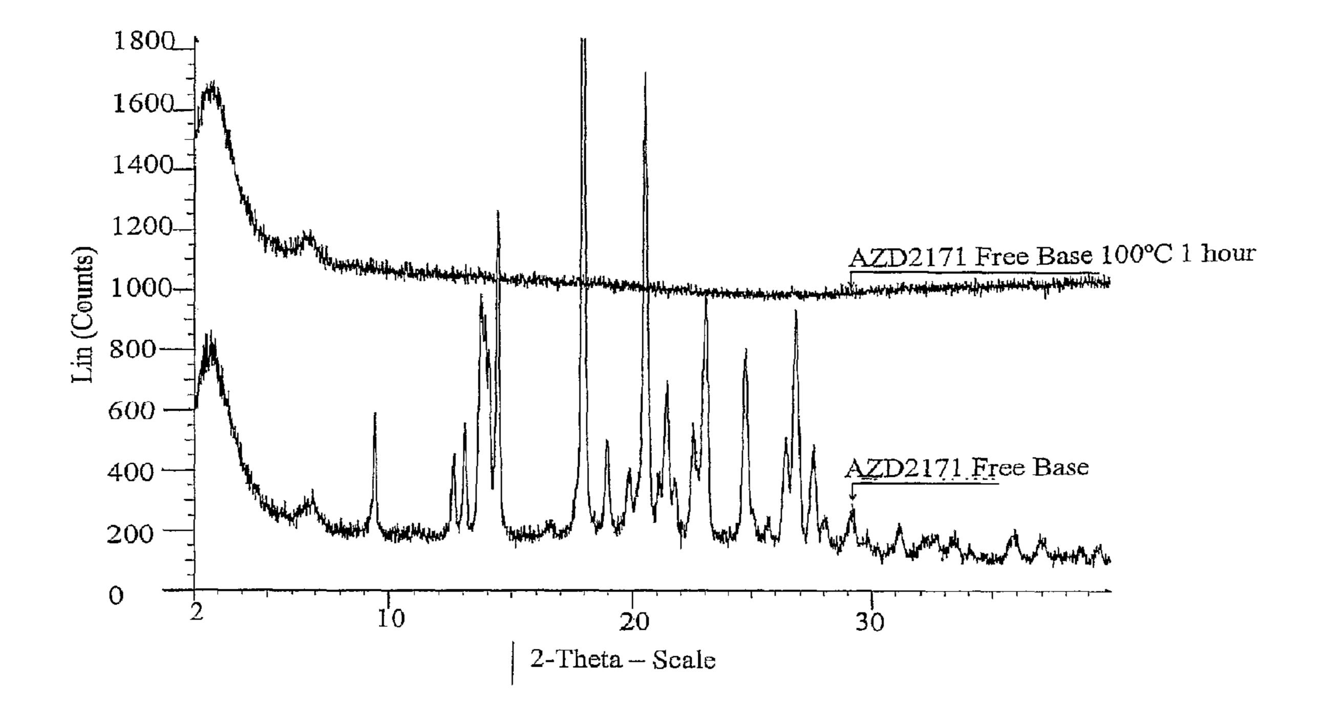
Figure 3: X-Ray Powder Diffraction Pattern AZD2171 Free base Monohydrate Heated to 100° C
