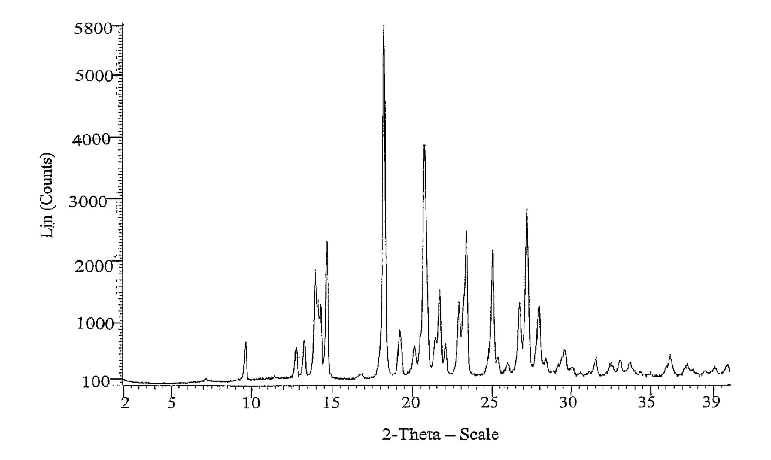
Figure 2: X-Ray Powder Diffraction Pattern AZD2171 free base
