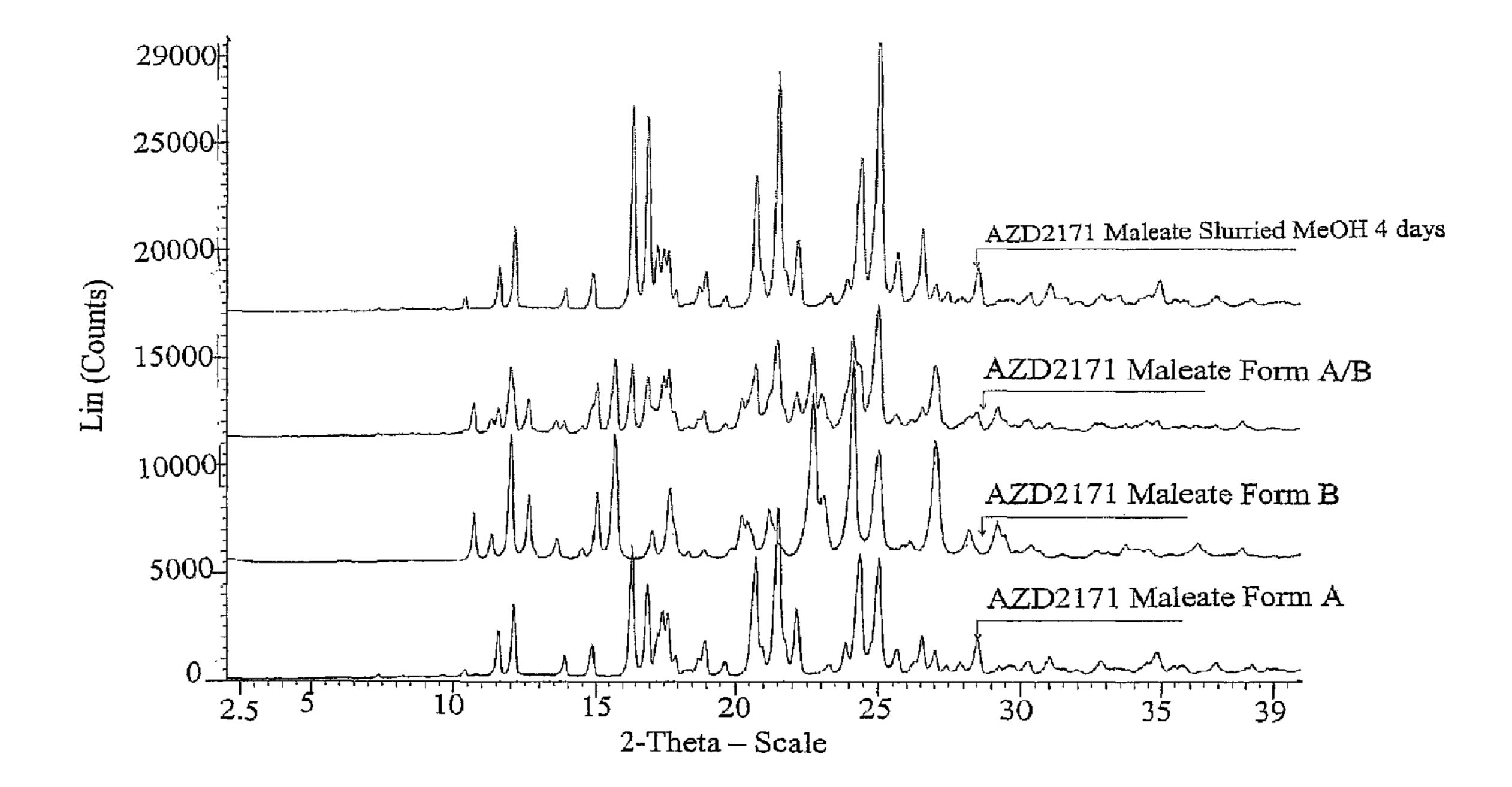
Figure 10: X-Ray Powder Diffraction Patterns AZD2171 Maleate Slurry Experiment
