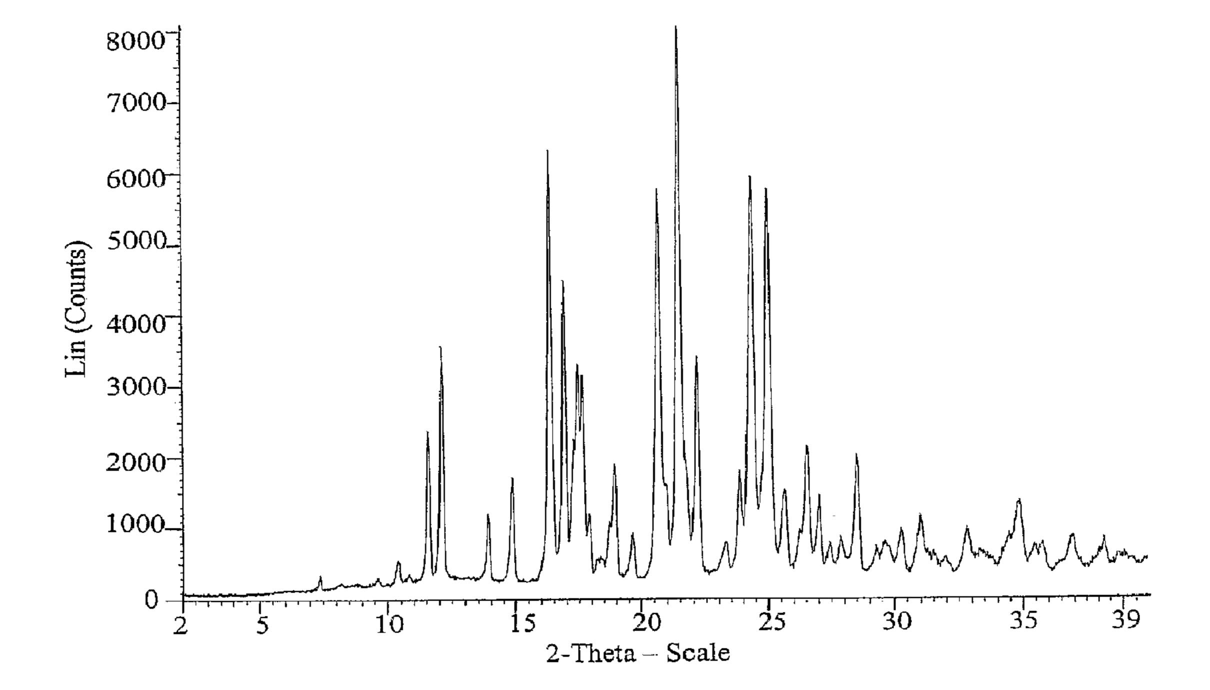
Figure 5: X-Ray Powder Diffraction Pattern AZD2171 Maleate Salt Form A
