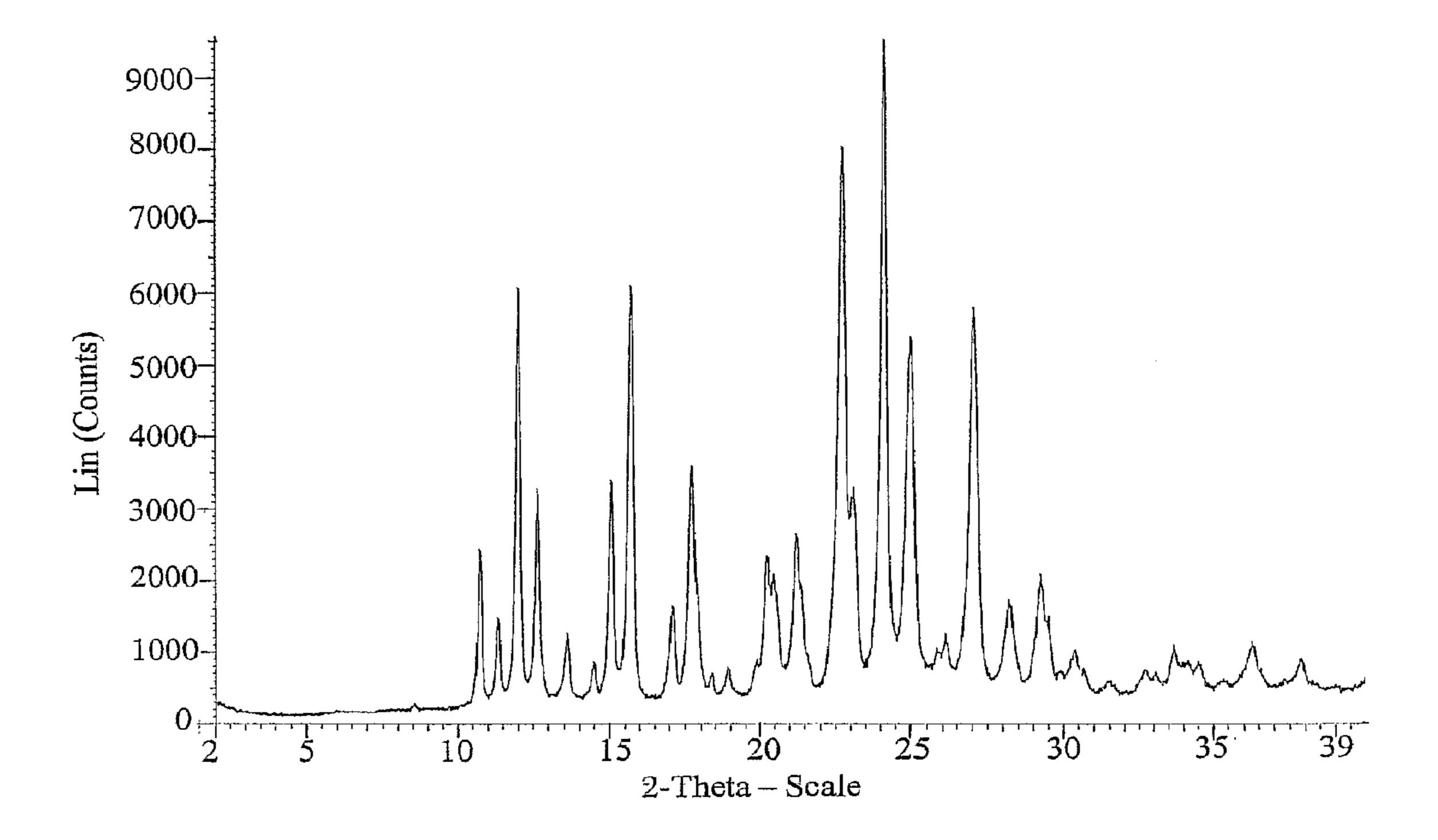
Figure 8: X-Ray Powder Diffraction Pattern AZD2171 Maleate Salt Form B
