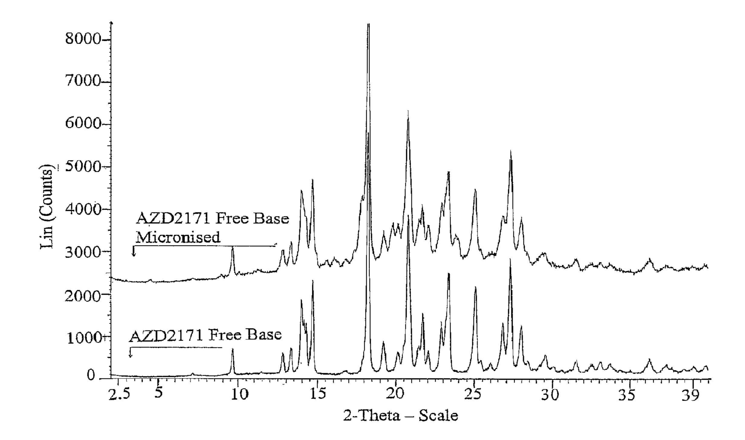
Figure 4: X-Ray Powder Diffraction Pattern AZD2171 Free base Micronised
