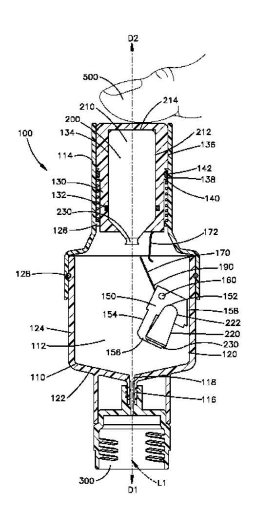
of the ampoule laterally and/or obliquely away from the central longitudinal axis to break the head of the ampoule from the body of the ampoule when the ampoule is moved in the first direction, removing material from the body of the ampoule, and removing liquid from the head of the ampoule.
