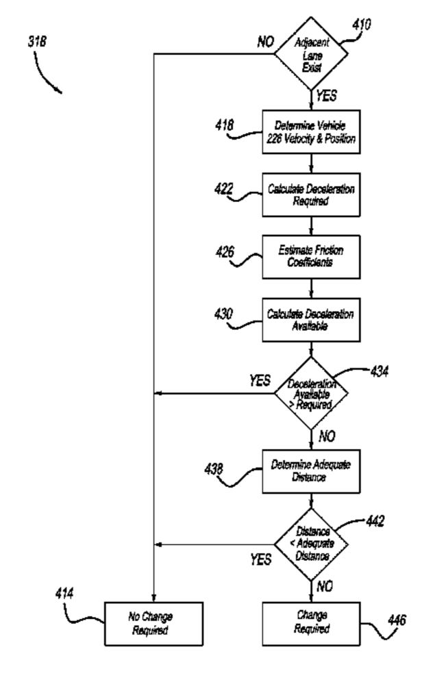
change maneuver based on the steering profile. The steering profile can include a plurality of steering angles and corresponding vehicle positions for maneuvering the vehicle from a current lane to an adjacent lane. The steering angles can be calculated to not increase the acceleration of the vehicle above an occupant comfort threshold value and to not cause the vehicle to cross an outer boundary of the adjacent lane.
