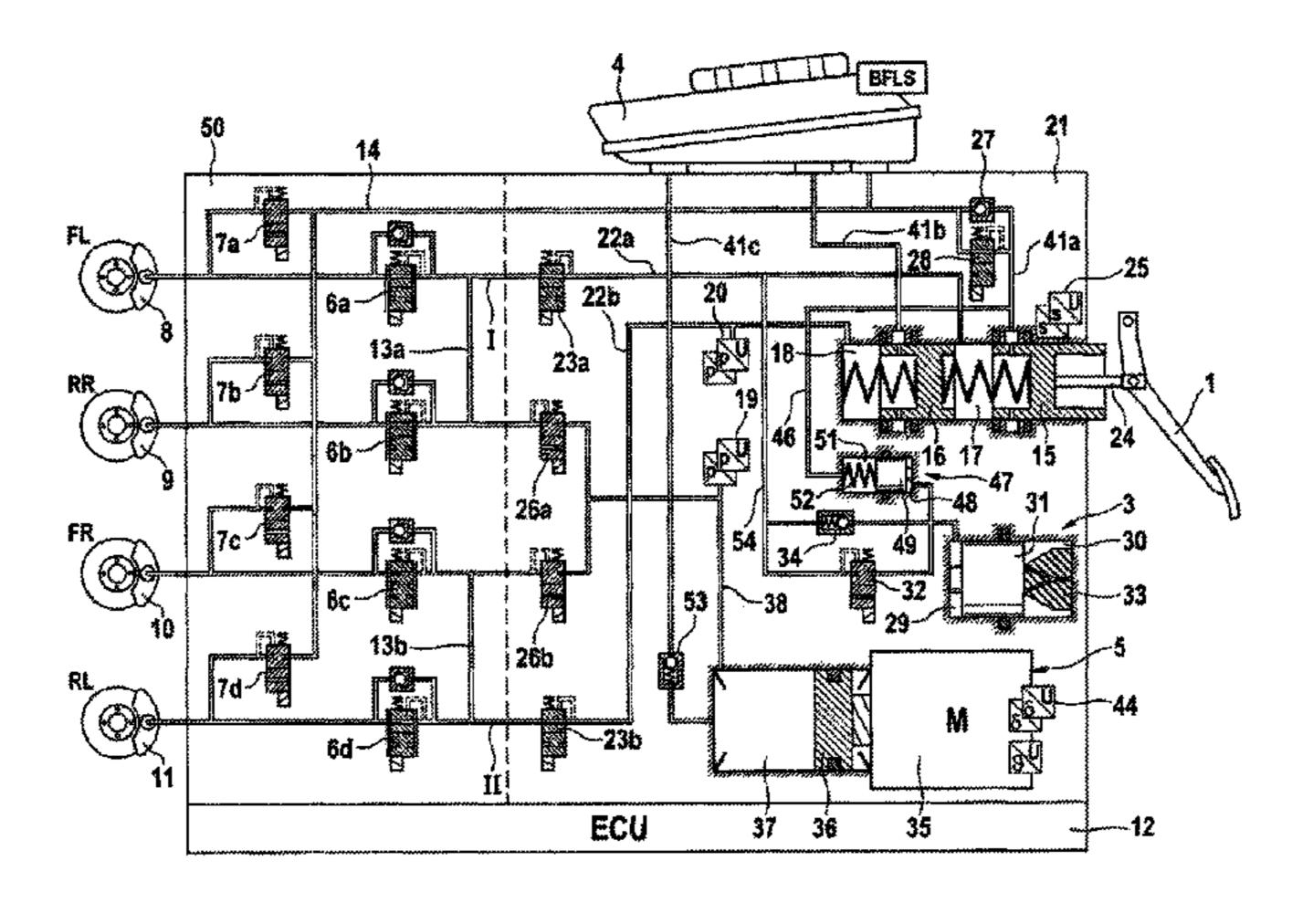
nected, or is hydraulically connected, through a first hydraulic connection (54) to the pressure chamber (17) and which has an electrically actuated isolation valve (28) with a pressure means reservoir (4) under atmospheric pressure. A media separator device (47) is arranged in the connection (46) between the simulator chamber (29) and the isolation valve (28).
