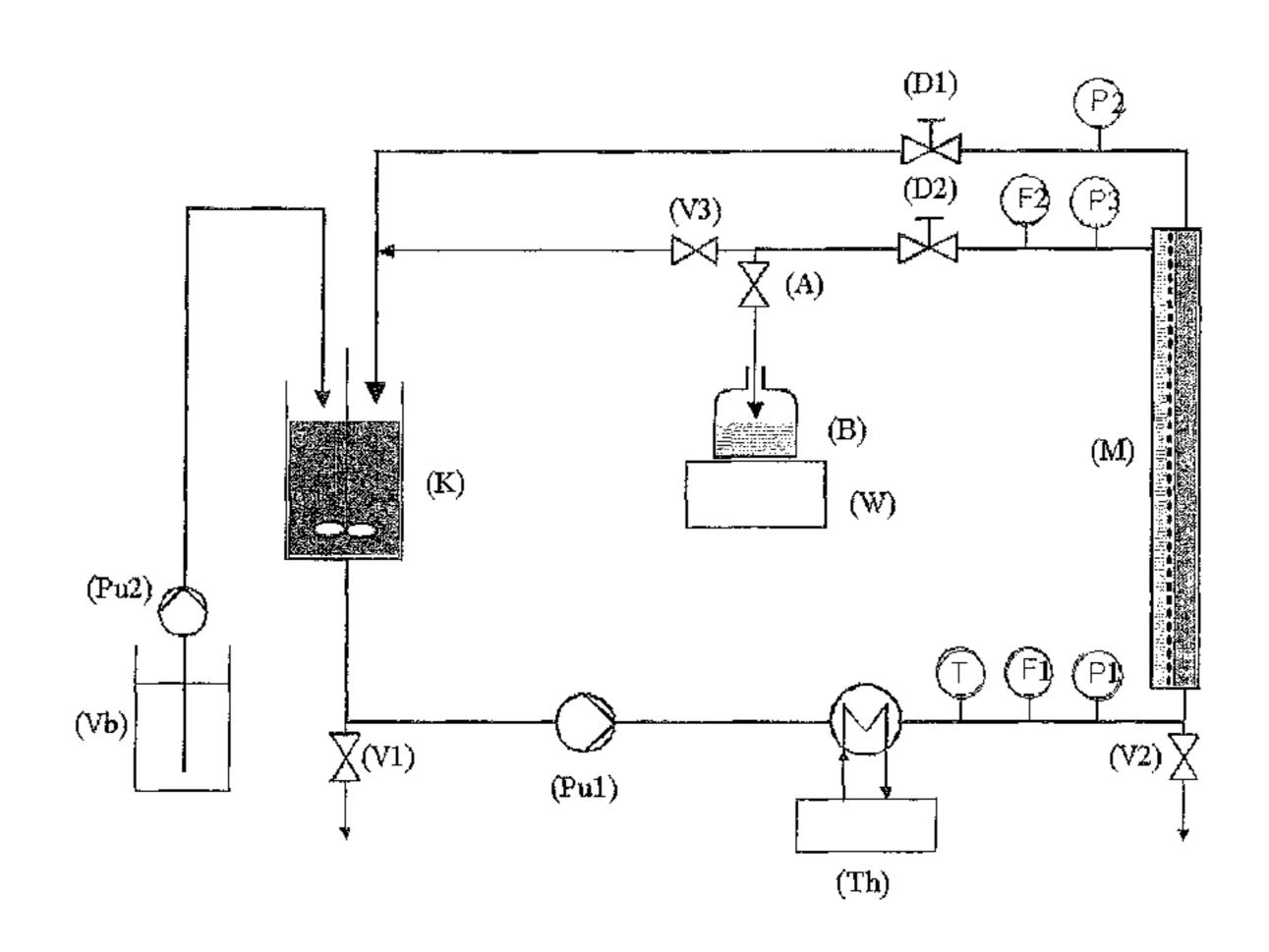
comprising reaction medium is taken from one or more reactors and the suspended, at least partially inactivated catalysts are separated off and purified by means of at least one membrane filtration, with at least one of the membrane filtrations being carried out as a diafiltration.
