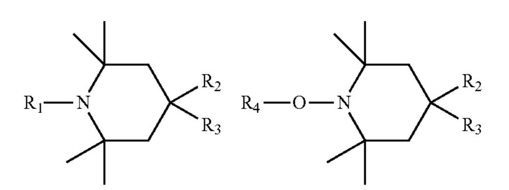
wherein  $R_1$  up to and including  $R_5$  are herein independent substituents; for example containing hydrogen, ether, ester, amine, amide, alkyl, alkenyl, alkynyl, aralkyl, cycloalkyl and/or aryl groups, which substituents may in turn contain functional groups, for example alcohols, ketones, anhydrides, imines, siloxanes, ethers, carboxyl groups, aldehydes, esters, amides, imides, amines, nitriles, ethers, urethanes and any combination thereof;
