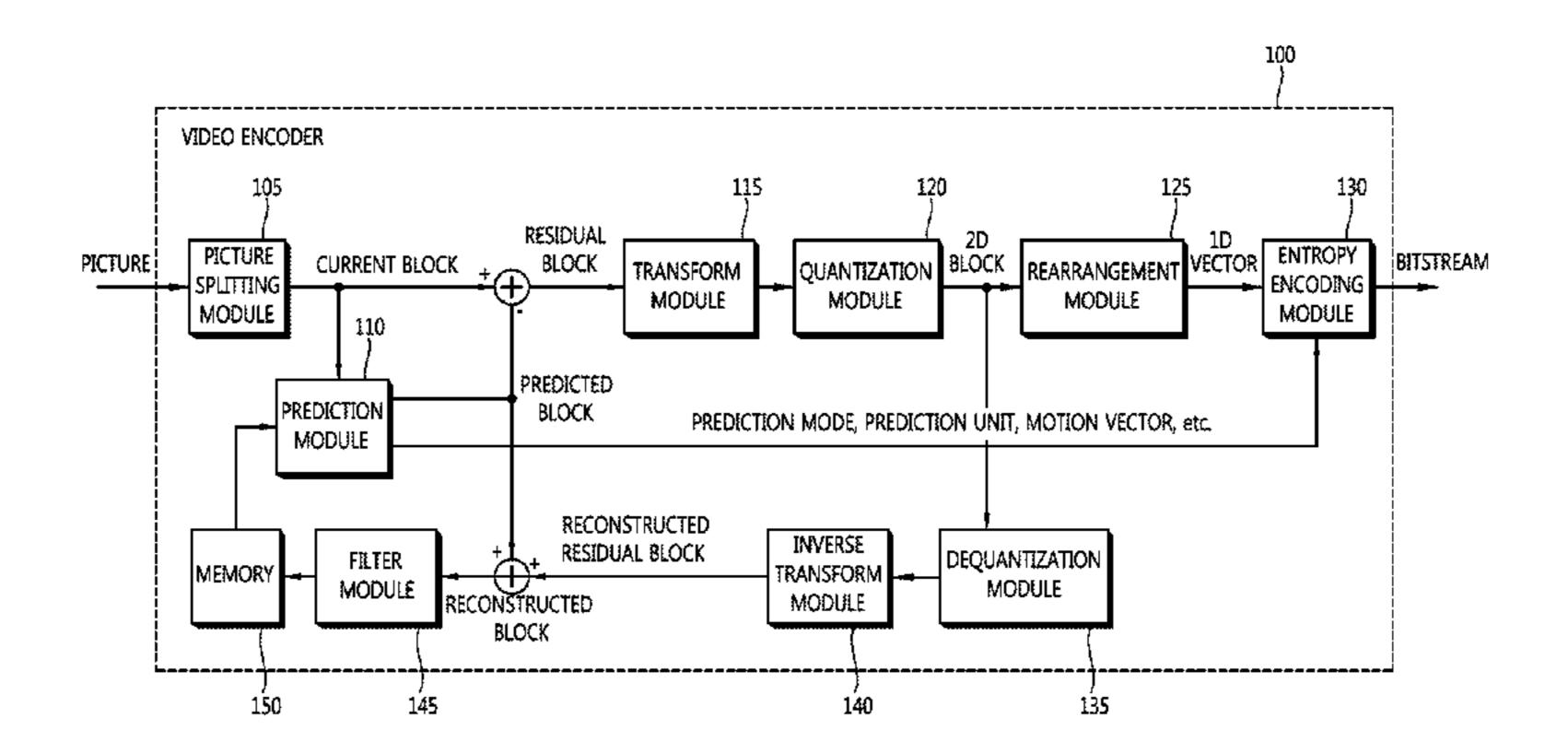
tion block corresponding to the current block by performing intra prediction for the current block based on the determined intra prediction mode.
