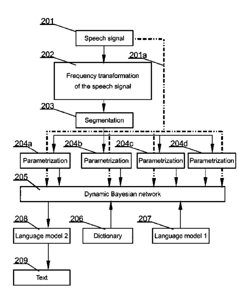
time-frequency domain (202) in at least two parallel signal processing lines (204*a*, 204*b*, 204*c*, 204*d*, 201*a*) for time segments distinct for each line, and analyzing in the analysis module (205) relations between observed signal features (308-312) for at least two distinct time segments in the analysis module (205).
