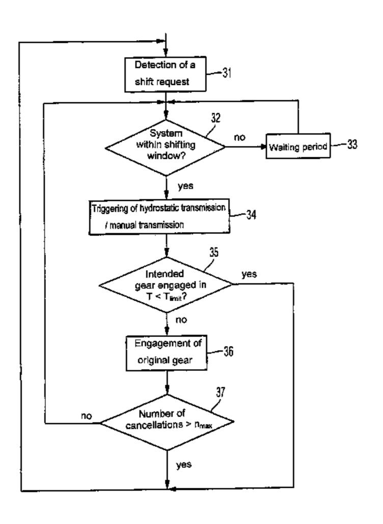
engaged through a gear stage change was successfully engaged is detected by a detection device, which is connected to an electronic control unit of the transmission arrangement. If the engagement of the gear stage to be engaged is not successful, the original gear stage is reengaged. After the engagement of the original gear stage, the downstream transmission is again activated such that the gear stage to be engaged is engaged.
