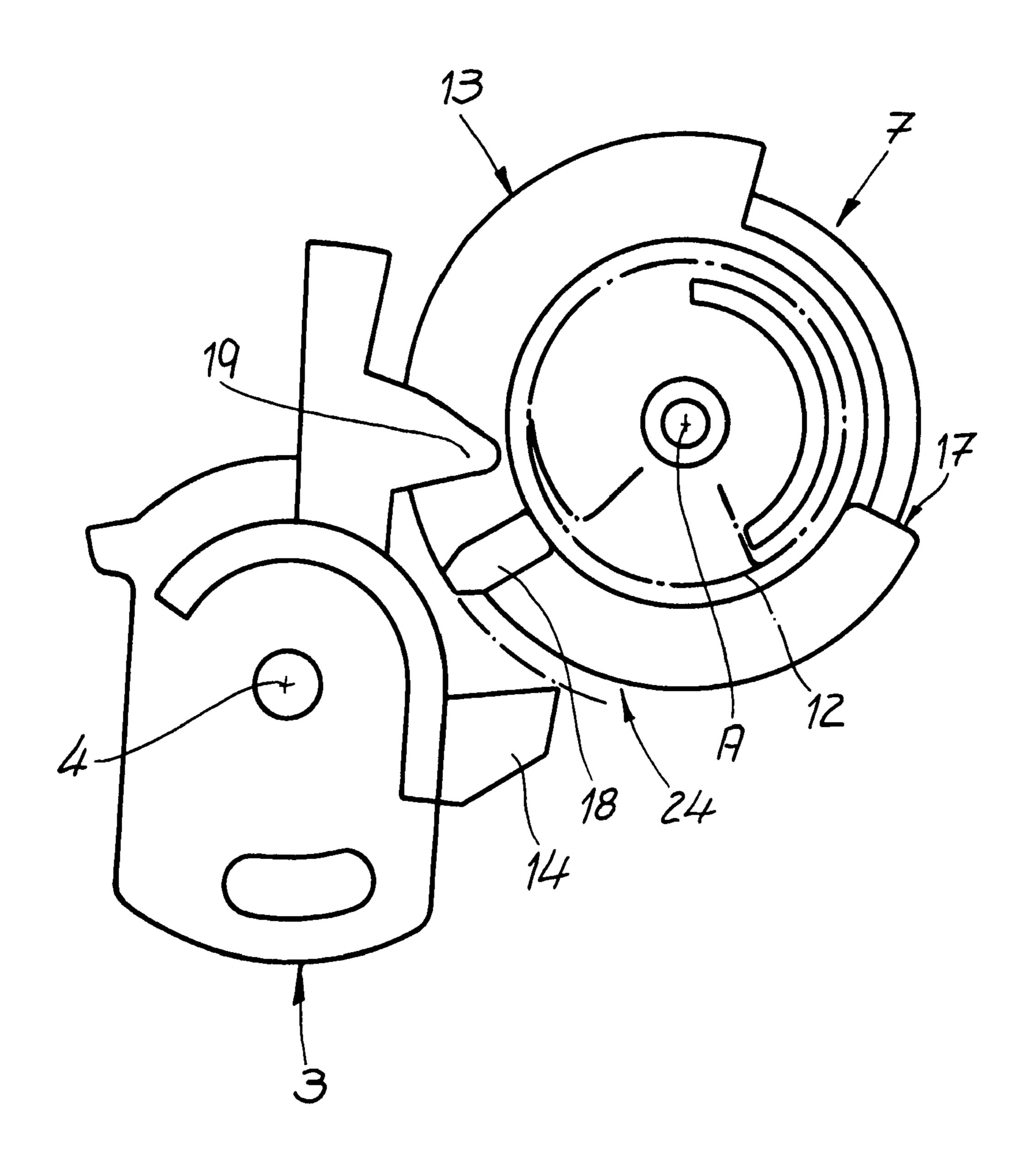
The invention relates to a motor vehicle door lock comprising a locking mechanism, at least one locking lever and an electric drive for the locking mechanism with the electric 5 drive acting upon the locking mechanism during normal operation for electric opening and also provides a mechanical opening of the locking mechanism at least during emer-
