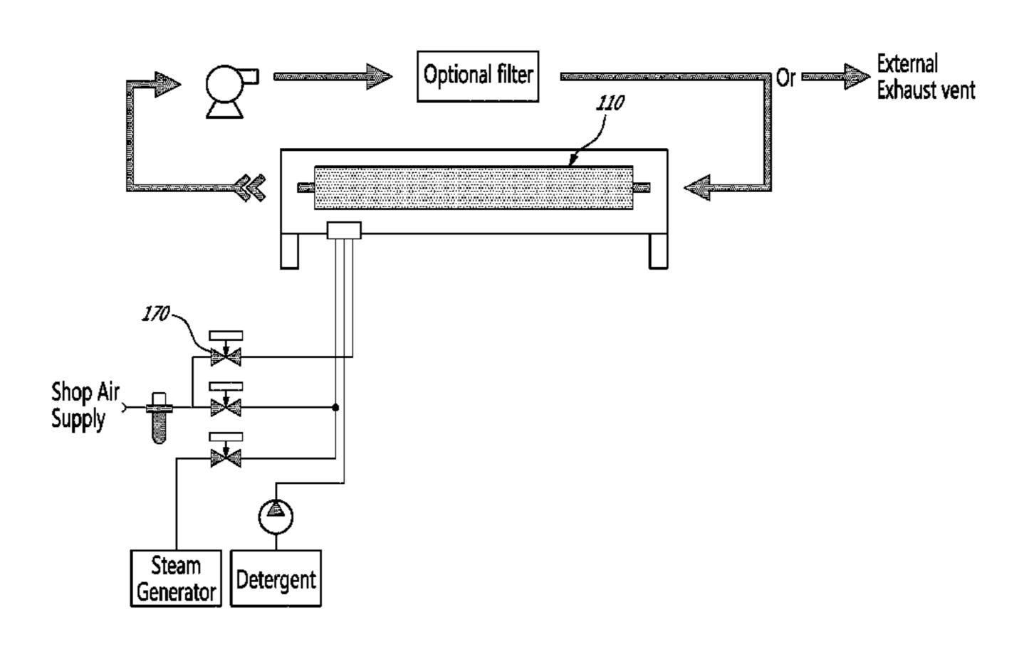
floors of printing units, the method comprising applying a detergent to the surface to be cleaned, after a period to allow action of the detergent, removing the detergent by rinsing, using a vapor and high velocity air stream, i.e. atomized water fog; or steam; or a combination of steam and air, which allows dislodging particles encrusted within cells of the surface of the piece of equipment to be cleaned.
