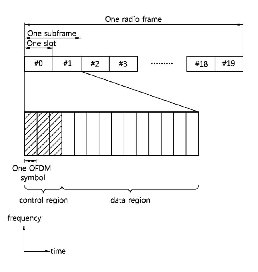
indication channel, and monitors the downlink control channel in the search space. The search space is defined by one or more pairs of physical resource blocks (PRBs).
