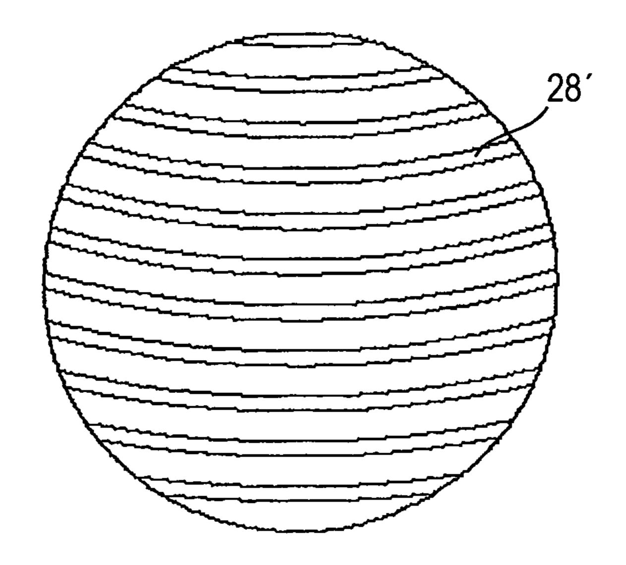
OPTICAL SENSING DEVICE FOR DETECTING AMBIENT LIGHT IN MOTOR VEHICLES COMPRISING A PRISM STRUCTURE HAVING A PLURALITY OF PRISMS DESIGNED TO DIRECT RAYS OF A SPECIFIC AMBIENT LIGHT BEAM
