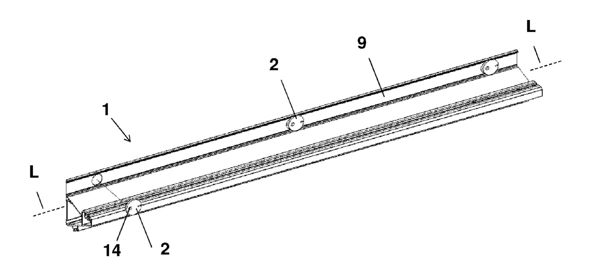
being non-uniform. The support bracket (1) has a support surface (12) adapted for engagement by the periphery of the support element (2). The invention also provides a method of mounting the support structure, and a support bracket for use in the structure and method.
