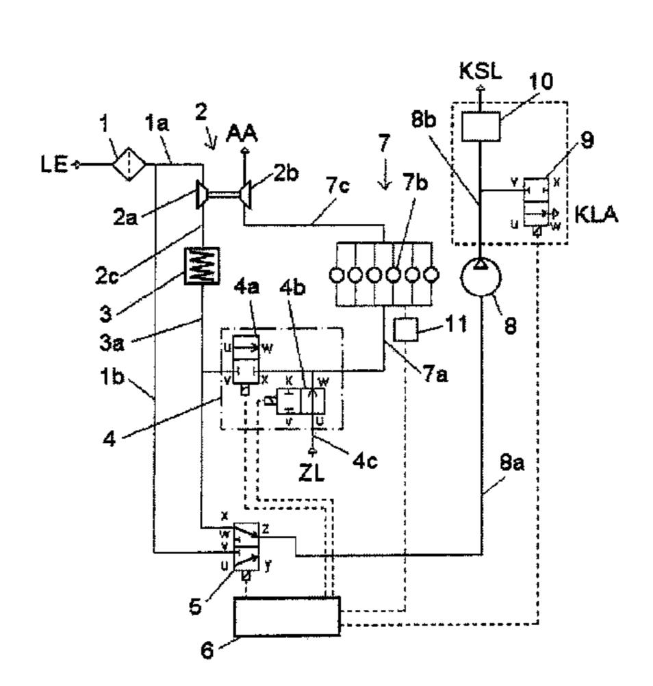
pressure-charged mode, the switchover valve switches the compressor from the pressure-charged mode into the suction intake mode.
