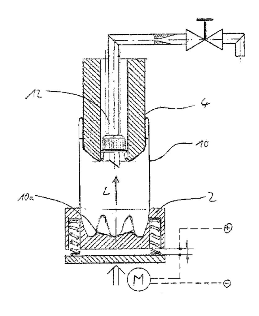
second region is arranged at a distance from the first region, with a removal device for removing liquid from the container and with a drive device which moves the second holding device in a pre-set direction of movement (L) with respect to the first holding device. The removal device is arranged on the apparatus in a removable manner and at least one element of the removal device is designed in the form of a one-way element.
