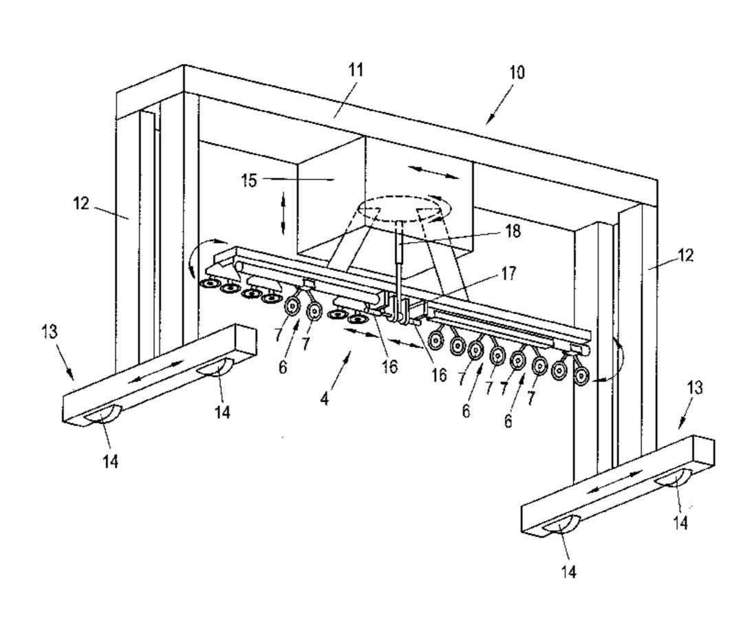
gripping device (4) suction heads (7) pivoted out of their operating position are arranged above the stacks (1, 2).
